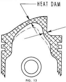
A piston dissipates heat by conduction to the cylinder walls and from then to the water in the jacket. In this process the heat is absorbed by the piston head, and if the piston is of good design, heat flows through the ring belt and rings out to the cylinder walls. When selecting a piston for racing, besure that there aren't 'any heat dams in the design of the upper section. A heat dam is a thin section that restricts the flow of heat just like a valve in a water pipe. Figure 13.
