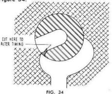
This is also the case with some flange rotors. A common practice is to bevel the corners of the indexing edges so that the blunt corner doesn't cause turbulence of the inflowing charge.
