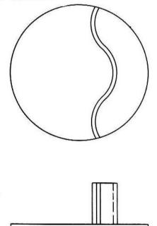
The purpose of the deflector is to keep the intake ports from discharging across and out the exhaust ports, and also to direct the charge toward the top of the cylinder to displace the exhaust which is left up there.
