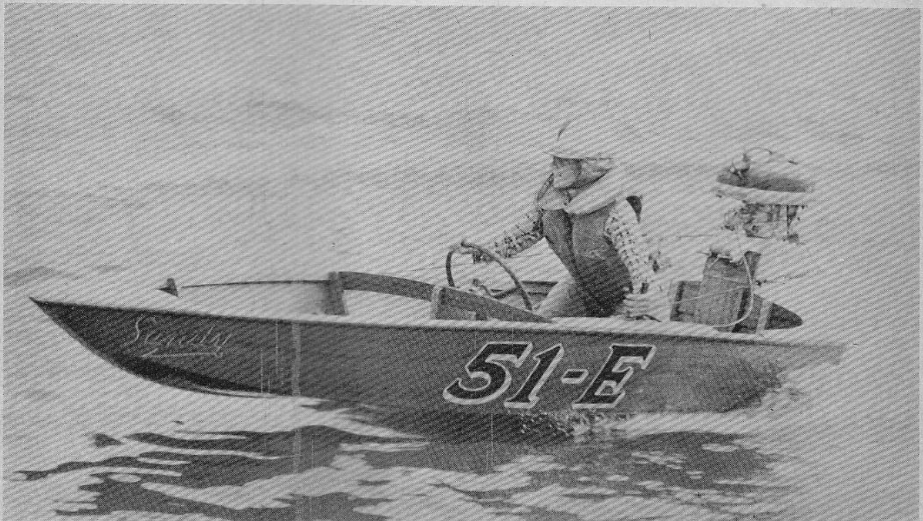
10 year old Doug Van Rossum, JU runabout "Sandy", Sid Craft hull. Mark 6 Mercury motor. Note the motor set up and the big smile.
