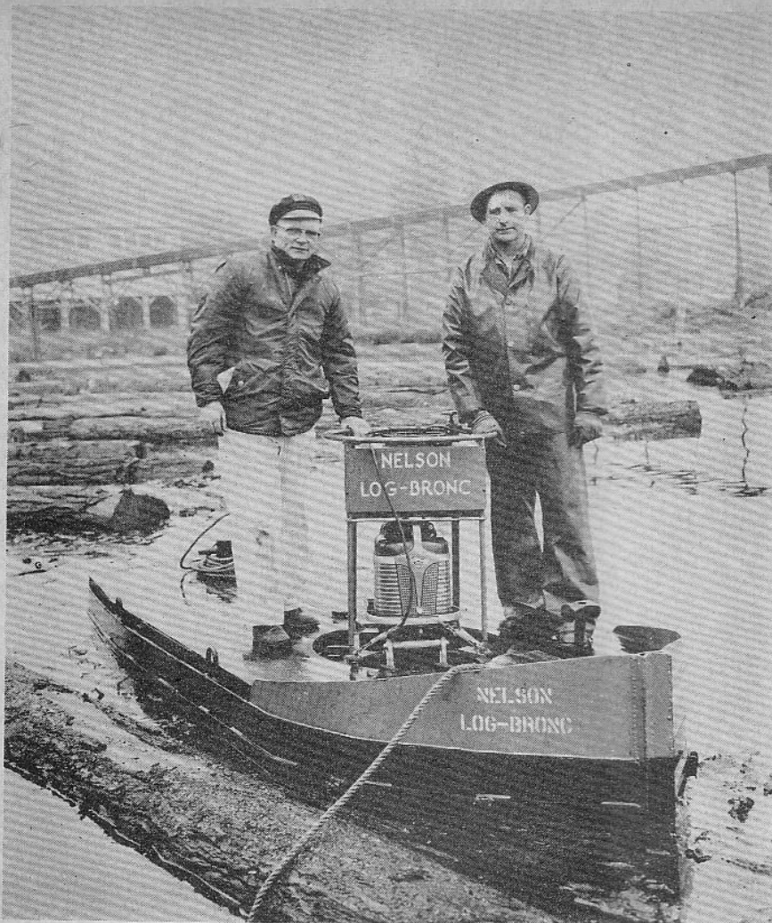
The Nelson Log-Bronc was invented by George Williamson of Coos Bay, Oregon to serve as a bulldozer in the log pond of a sawmill. Bert Miller of Coquille, Oregon was the skipper of the first Bronc.
