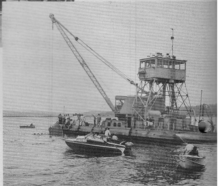
The rescue operation for sunken boats was the best ever. A team of Navy lung divers went down and attached the slings to the sunken racer — then the C.G. derrick barge brought them gently to the surface. Here "Rebel Suh" comes off bottom.
