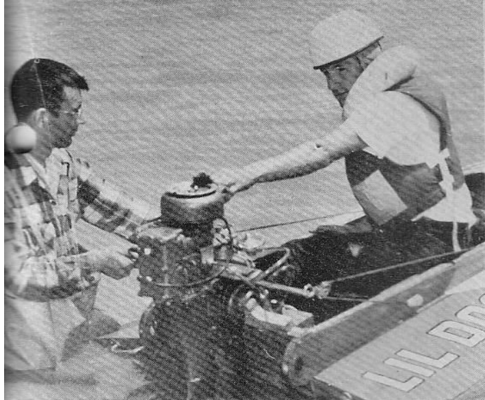
Conventional rope starting, weight is saved and price reduced without re-wind starter.
