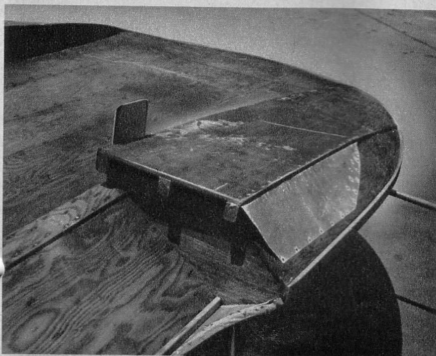
The sponsons have been changed a dozen times and probably aren't right yet . . . Hence, we use a quick change system like the one illustrated. Note fin placement.
