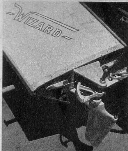
Closeup of the Debbold rudder assembly and all necessary fittings. Both cables from the quadrant run along the left side of the boat under the decking. Note speedometer takeoff at the top of the rudder.
