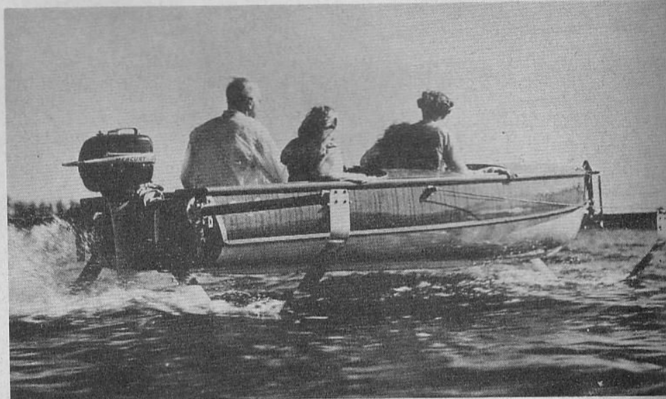
American industry has led in the development of the use of hydrofoil "legs" for the outboard runabout. Installed on a standard boat powered by a Mercury motor with extra long drive shaft, lightweight duraluminum hydrofoils lift the craft about 18" above the water at high speed. With a full load of passengers, the hydrofoil equipped boat will cruise at about 35 mph with the motor operating at only half throttle. Safe turns can be made with very little banking. This design is built by the Baker Manufacturing Co. of Evansville, Wisc.
