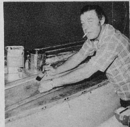
Step No. 2. Applying more resin.
