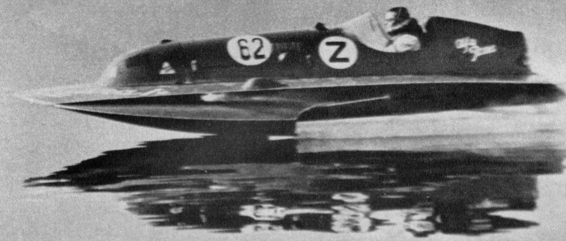
Verga's Laura prop-riding in perfect trim at 140 mph — perfect mile trial water too.
