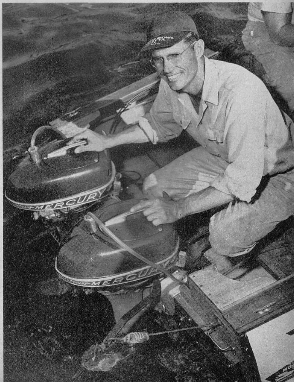
The Marathon winner. Note the steering arrangement. Each of the Mercury Hurricanes has a steering bar on the outboard side, as shown in the photo. A chain couples the two motors so that they turn together when the steering wheel is turned.
