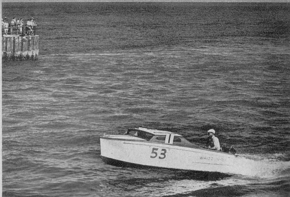
The Marathon winner. Note the steering arrangement. Each of the Mercury Hurricanes has a steering bar on the outboard side, as shown in the photo. A chain couples the two motors so that they turn together when the steering wheel is turned.
