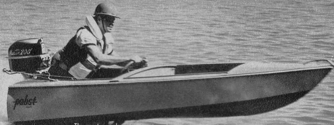
The most popular of all racing classes—the B Stock Runabout. Here it's a new Martin Silver Streak in action driving a Pabst "B" hull. This motor is eligible for racing in B stock class.
