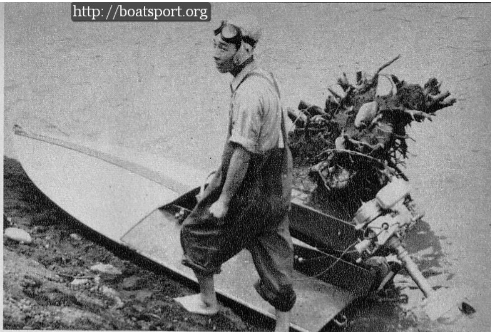
Mr. Ataka the driver for H. Ito of Kinuta Motors Co. Hull: Sumidagawa Shipyard Co., Tokyo. Motor: Kinuta Class B—20 cu. in.—16 h.p. at 4500 rpm, internal rotary valve—maximum speed on conventional Hydro 46 mph. Note: Lower unit—copy of old style Johnson KR55.
