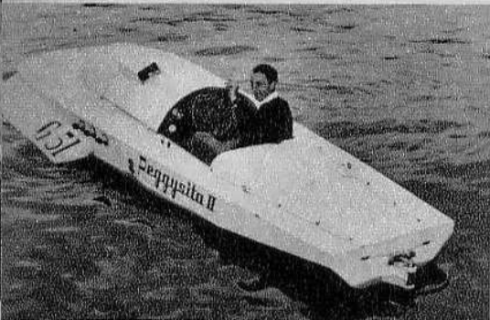
Raleigh Gibson's new 266 Hydro Peggy-sita II. Built from Champion Boat Plans—equipped with Smith and Jones heads, cam and reworked valves—Vertex Mag-neto and Hilborn-Travers Fuel Injection.
