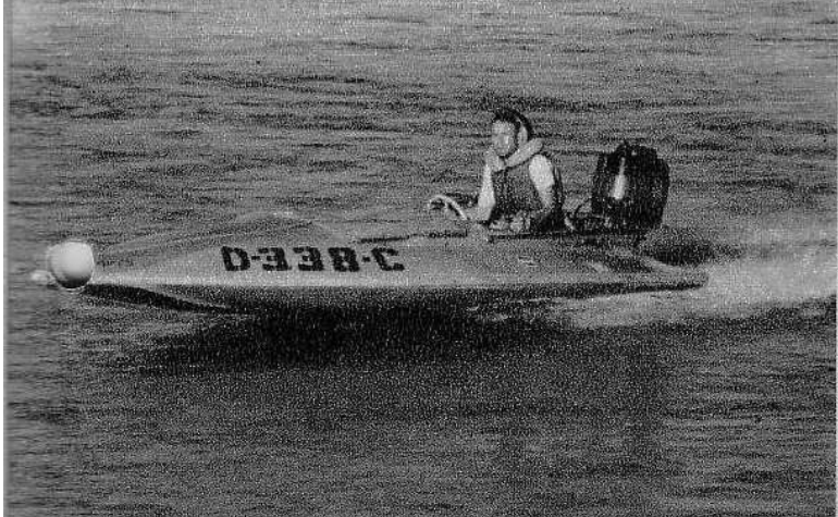
What is it? A Hydrabout or a Runaplana? Mike Davidson's all fiber-glass outfit. It looks like a hydroplane but measures to the 1951 APBA Stock Runabout specifications . . .
