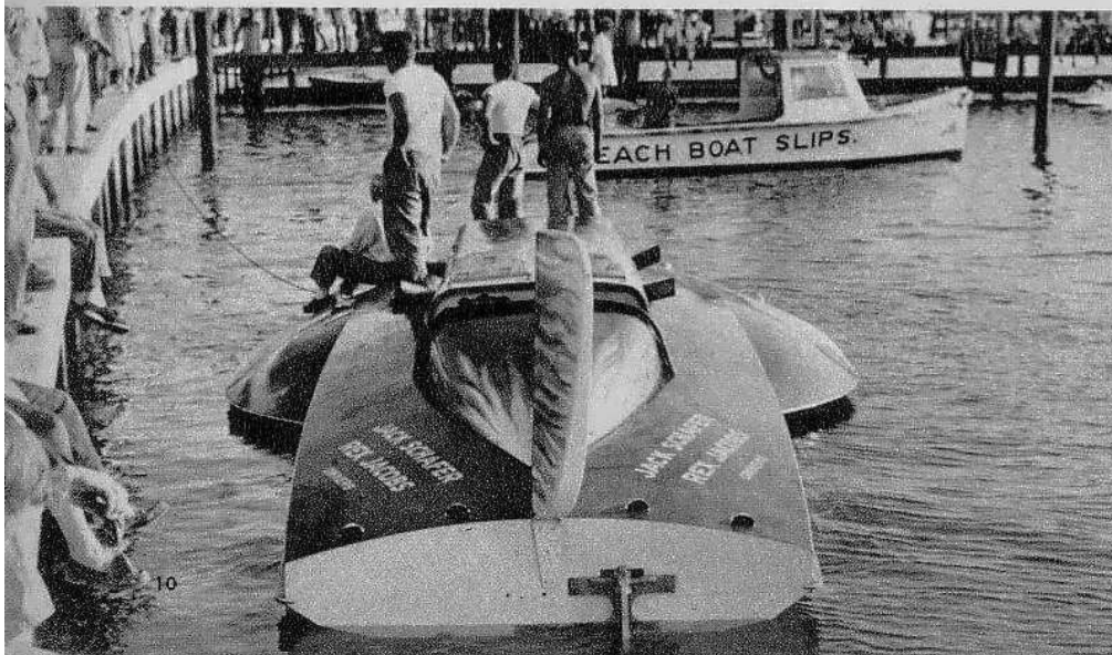
IN THE WATER . . . Offset rudder assembly with drive from power steering thru transom. Trim tab of stabilizer fin set at extreme angle to correct torque which developed in trials.
