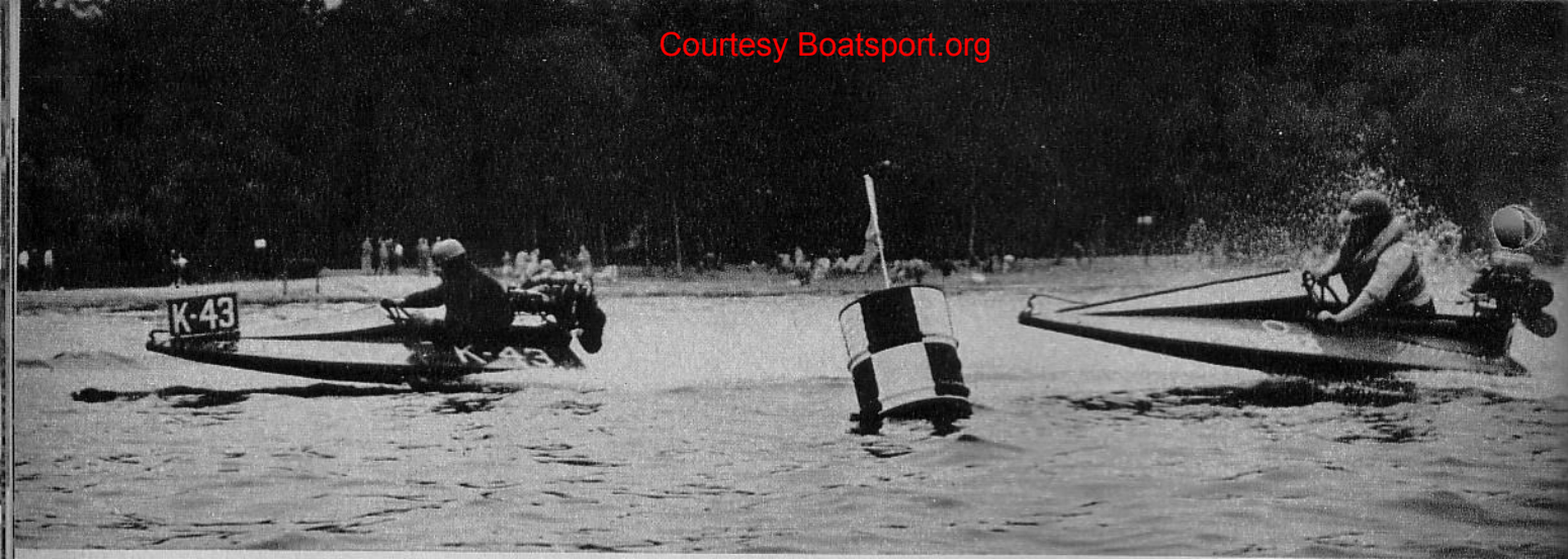
Ken Taylor in Tsetse (K43) winning the Watsonian Cup at the B.O.R.C.'s Ruislip meeting. His engine is a converted 500 cc J.A.P. Speedway motorcycle unit.
