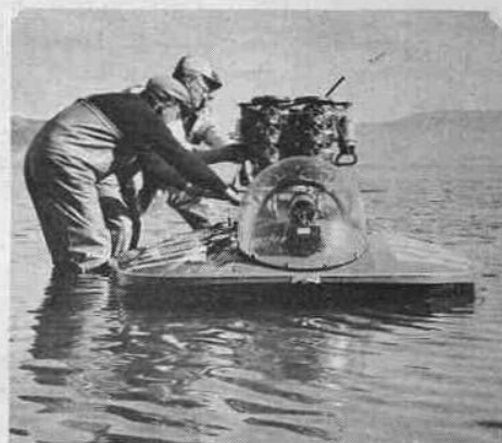
Long, Hren and Fife check over the motor fastenings before test run. Gadget forward of steering wheel is Sun Electric tachometer.
