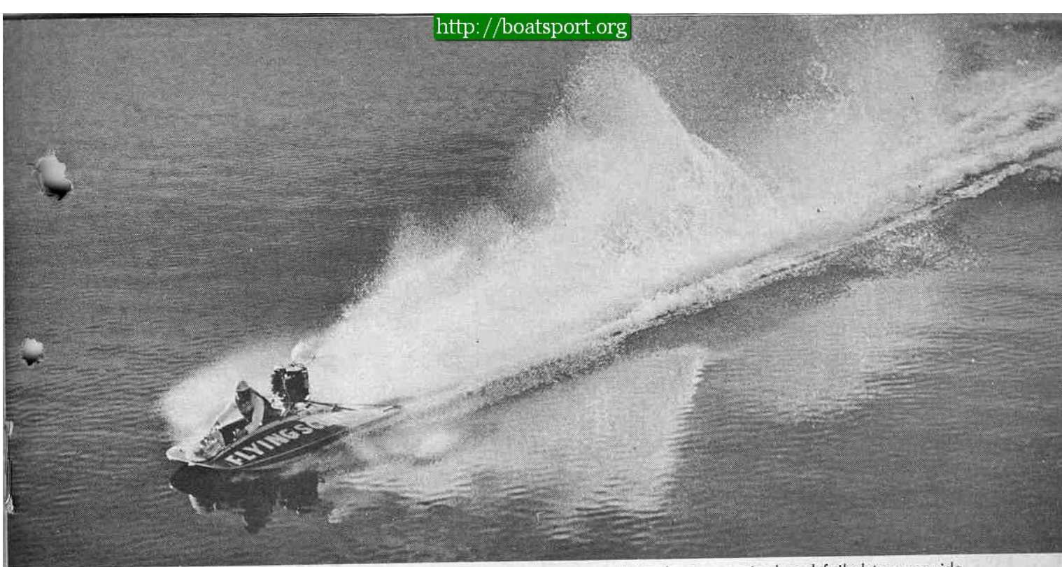
On this run, the planing angle of the sponsons was wrong and the boat porpoised and failed to prop ride.
