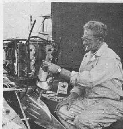
Lower unit overdrive gear was thirsty. Louis Hren is feeding it gallon and half of SAE 90It oozes away in short order.
