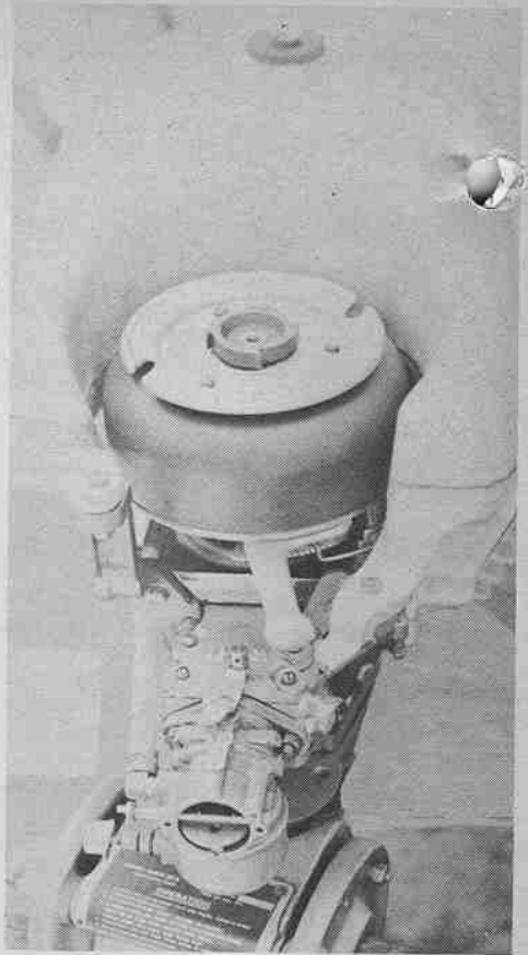
Left: The Jet Pac, made by the Ray Alberty Co., is designed to give a 15 per cent hp boost to 35 hp Johnson, Evinrude and Buccaneer motors. The full kit costs $49.95.
