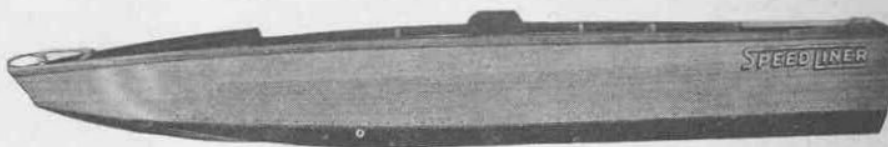
This Speedliner M-510 Corsair is 10 ft. 6 in. l.o.a. with 47 in. beam. It weighs 110 lbs, and costs $335. Other competition models run from $195 to $445.
