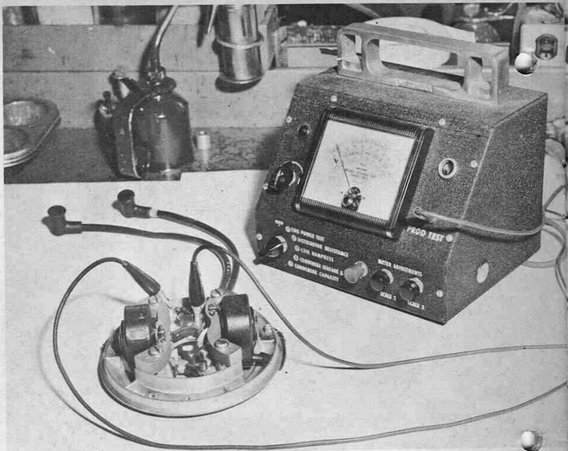
Testing a magneto for high resistance in the primary circuit with the new magneto analyzer. It will reveal whether the condenser is improperly grounded to the stator plate.
