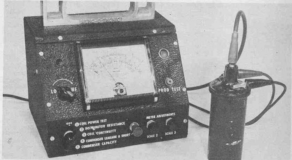
Automotive type coils can also be tested for maximum amperage, surface insulation and the like.
