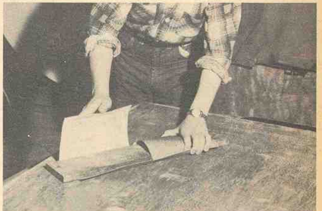
A large flat iron plate is ideal for sanding the stern section flat. Use an open-cut garnet paper, medium grade, for this part of the job.
