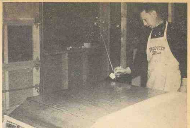
Resin is applied to half the bottom at a time. After the cloth is laid back over the stern, the forward half is treated in the same manner.
