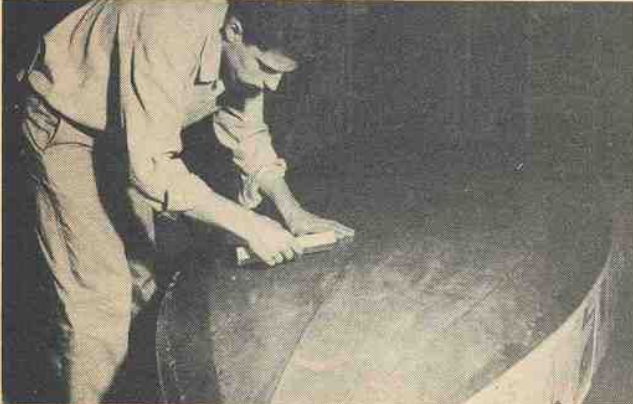
The entire bottom has now been covered with resin, and the cloth laid over it. More resin is now applied over entire surface with a squeegee.
