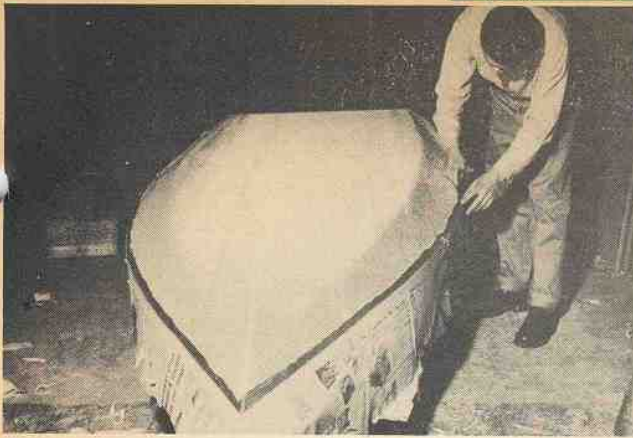
The fiberglass is laid over the hull bottom and trimmed to size. This is boat-cloth grade and it trims well; notching in front is unnecessary.
