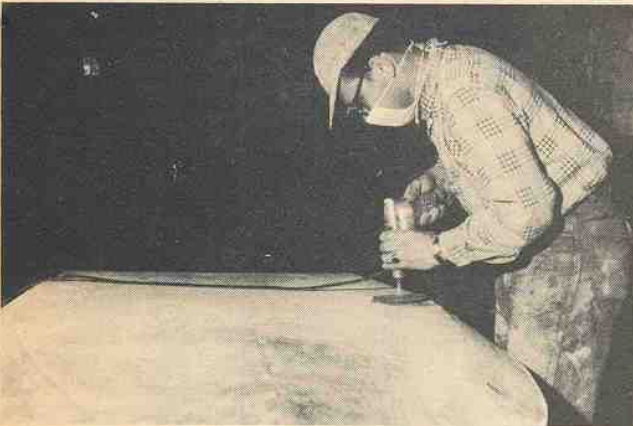
All large bumps are ground off with a disk sander. Don't cut into the cloth, except at the edges, where it must be feathered into non-trips.
