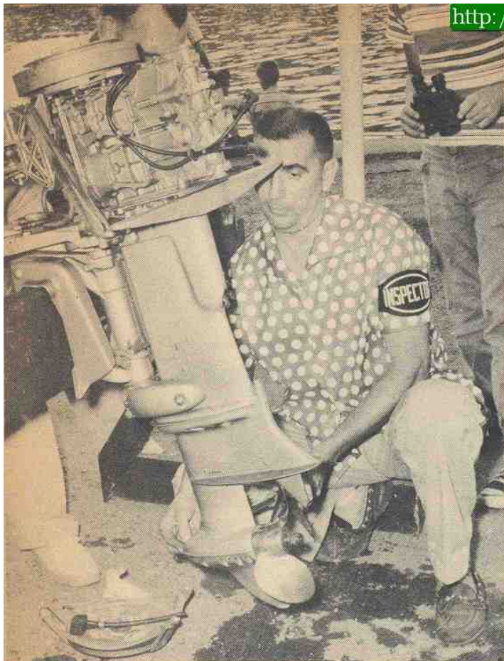
Each competition lower unit must meet a set of specifications. Inspector Larry Teel checks to see that the "Q" dimension has not been lengthened.
