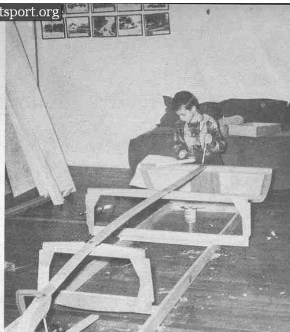
The builder pauses to read instructions. The first stages have been completed, with two main frames, keelson, stem and transom in place.
