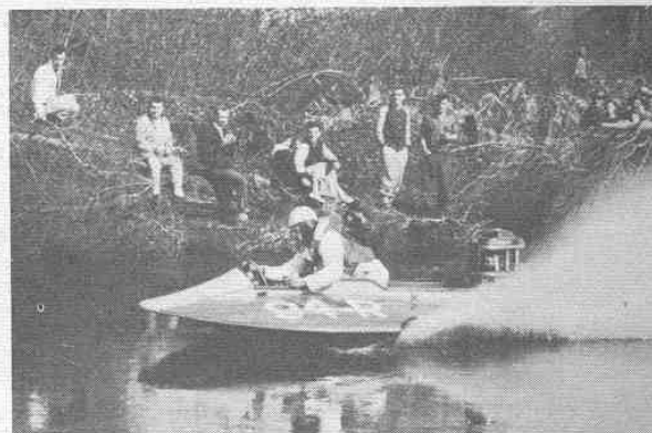
Cabover-design hydro places driver farther forward in the cockpit than traditional three-pointer. Design functions well with lots of power.
