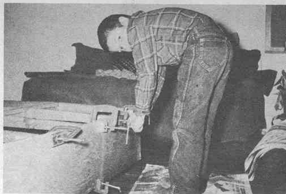
Wood blocks were placed between the clamp jaws and the wood to be held to prevent the surface of the wood from being disfigured or dented.
