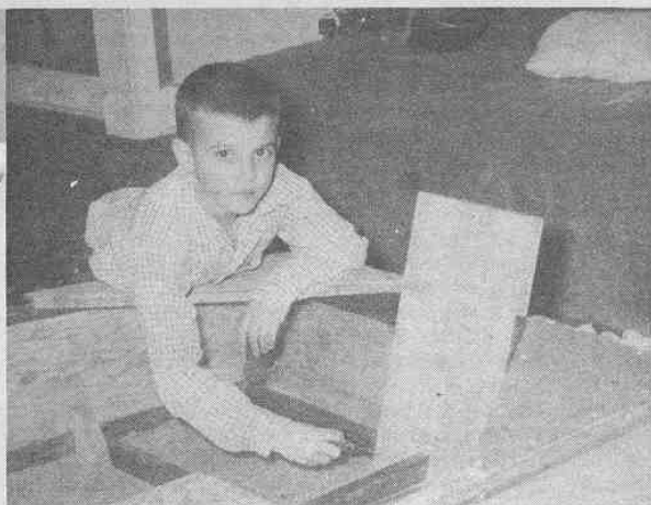
The last screw is set and the boat is ready for sanding and painting. Inaccessible spots had been varnished before they were covered over.
