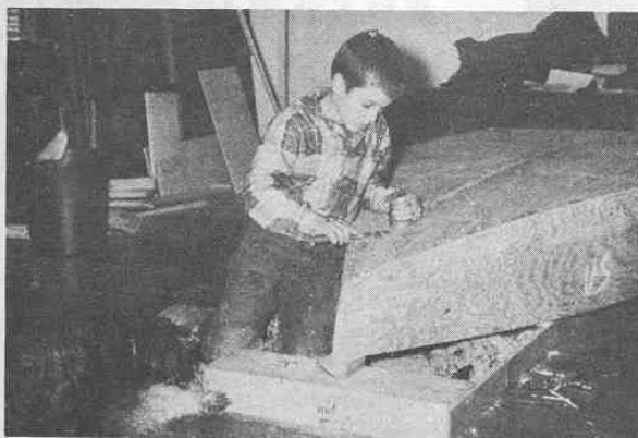
Bottom planking was screwed into place, all screw holes were countersunk, and holes were filled before the boat was finally turned over.
