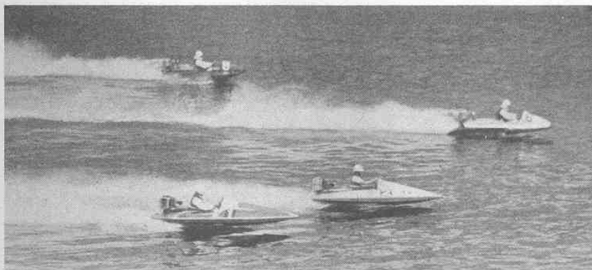
In Europe, heavy Class X motors are run on sit-down type hydros. Cockpit location of two boats farthest from camera resembles our cabover designs.
