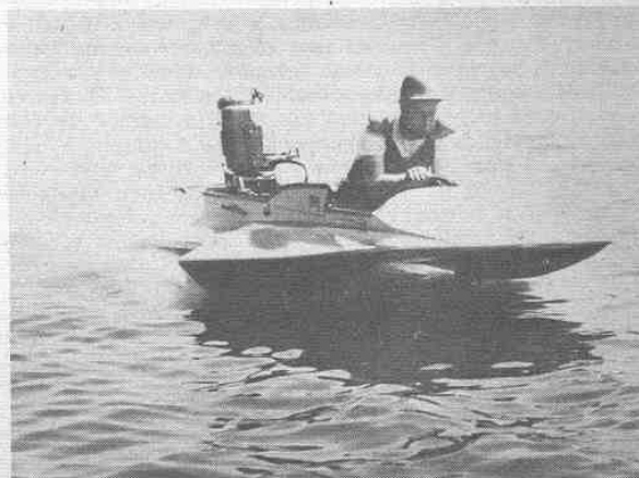
Front quarter view of a Record cabover design illustrates how, even with outboard hull, mass of the boat's area is forward of center of gravity.
