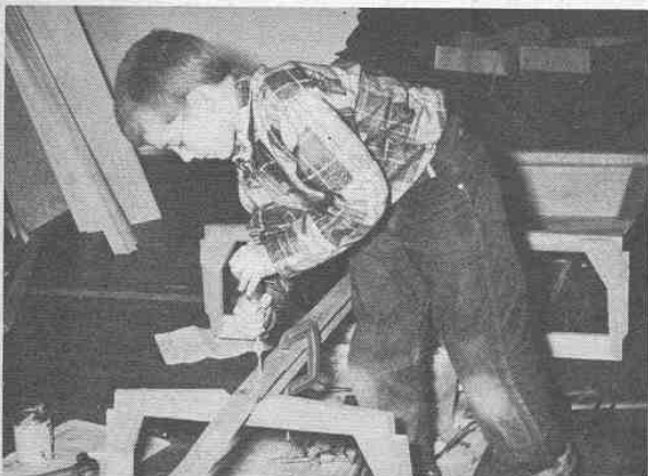
Clamps were used to hold the inner keel sections until the screws had been set with ratchet-type screwdriver. Craig needed little help here.
