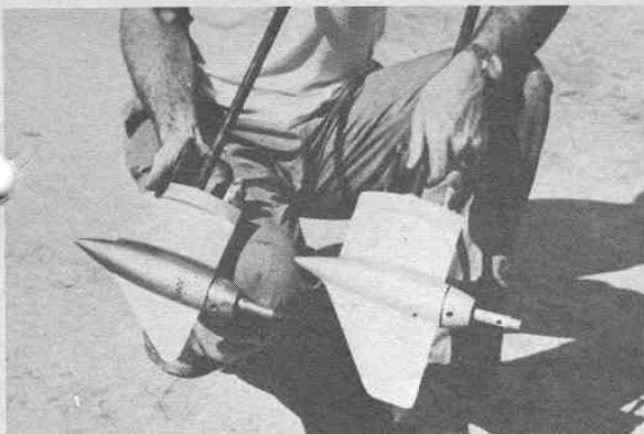
Contrasting two lower units made for same model motor: unit at right has different water intake; deeper skeg permits higher transom mounting.
