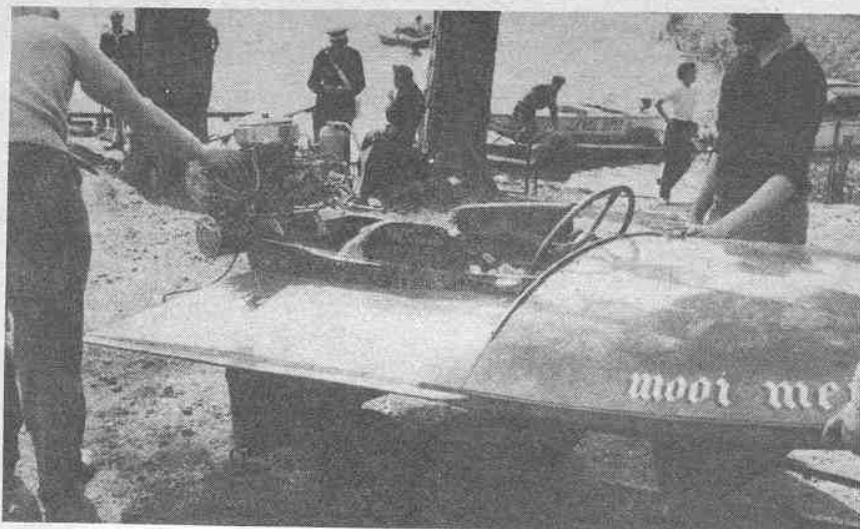
Charlie Trumper's Mooi Meiste formerly raced as Thunderbolt in the hands of Len Melly, one of the fastest of England's drivers. Note the unusually wide short hull for a single-step design.
