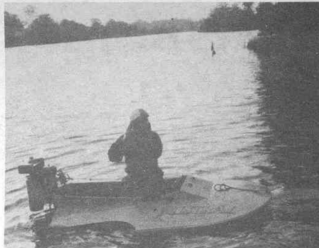
Mistral is a McCrae 3-pointer built last winter by her driver, Alan Richards, fast despite the old, inefficient Anzani motor.
