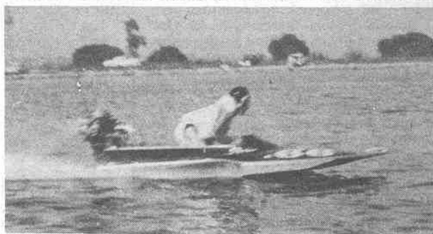
Set up for competition and short turns, Hubbell-Sorenson hybrid can run about 62 mph. Straightaway potentials indicate possible new records.
