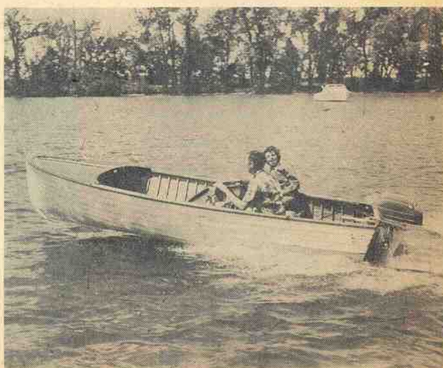
This 15-foot runabout by the Lyman Boat Works has a 64-in. beam and a 54-in. transom width. The 330-lb. boat has four seats, carries up to 750 lbs., and will take an outboard up to 40 hp. $470 F.O.B. factory.
