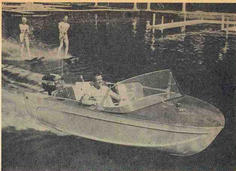
This is the smart Fleetwood in the Switzer Craft line, a very successful 15-footer with 74-in. beam and 34-in. depth. The 6-passenger craft weighs about 295 lbs., and takes a maximum load of 820 lbs. The Fageol V.I.P. engine can be factory installed to order.
