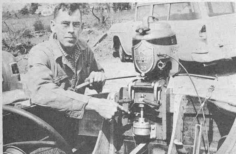
Williamson points to hydraulic lift on his Sid-Craft. Piston is extended and motor raised on sliding transom bracket. Two-inch variation is permitted by piston movement.
