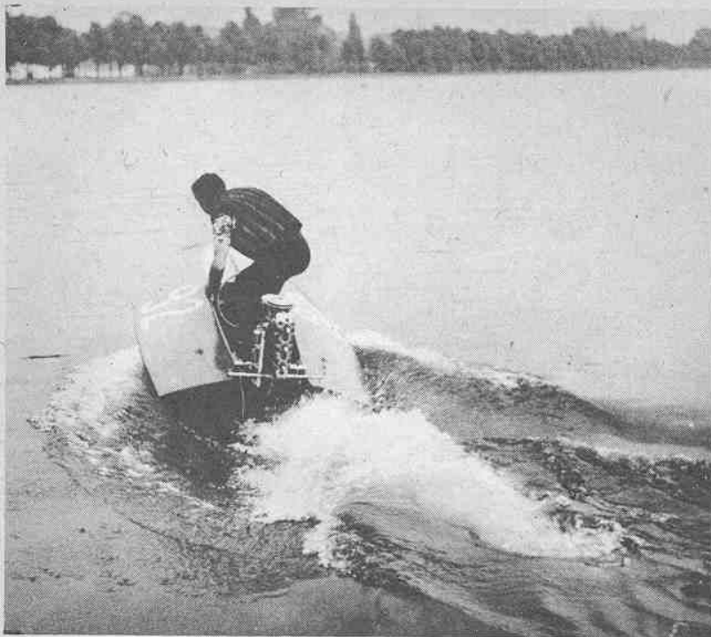
Twenty-six-year-old Dieter Konig, son of firm's founder, testing a three-cylinder-in-line C racing motor on conventional-design European hydroplane.
