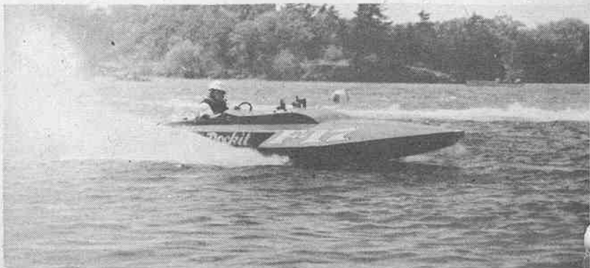
The 266 c. i.'s can burn methanol fuel in competition or mile trials. Motor cost must not exceed $1250 and hulls must be at least 16' long. Mile straightaway record is 121.703 mph.
