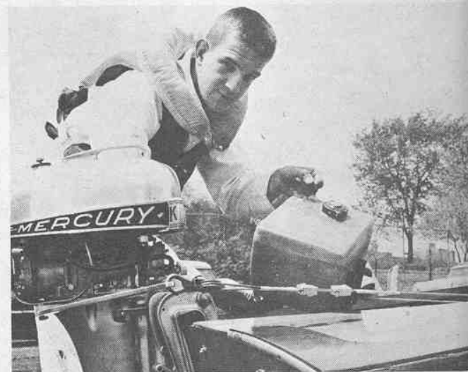
Rand Hippler, Detroit, who drove a Rinker to fourth spot in AU at Belle Isle, demonstrates a lightweight plastic fuel tank he constructed of fiberglass and designed to fit contour of his boat.
