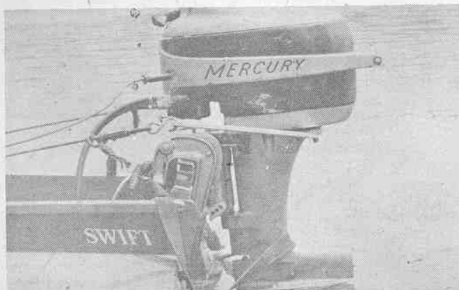
Maximum speed was reached without permanently building up the transom at 16 1/8 inches, when 58 1/2 mph was hit, and no slippage was evident.
