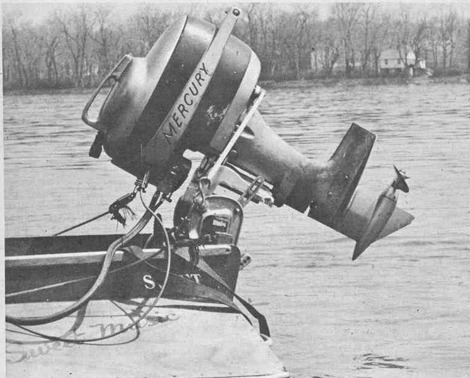
With the transom jacked up to 15 1/8 inches and using the old style 20H unit with a #23636 propeller, Larry Teel clocked a run at 56 mph.
