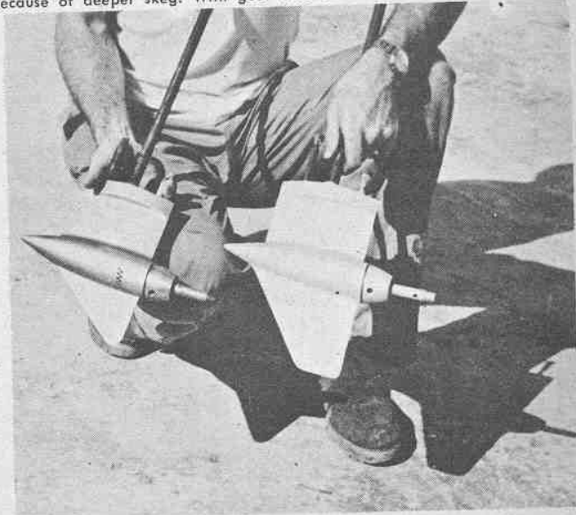
Comparison between skegs of old and new units is clear in this view.
