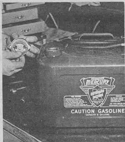
Remote fuel tank should get attention. Make sure that the gasket on filler cap is in good condition and fuel line fittings are tight.
