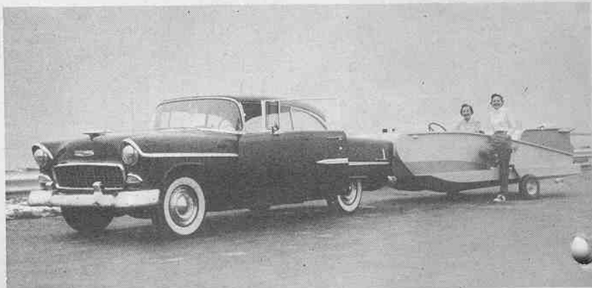
The Nomad is a semi-catamaran type craft which carries its own trailer. The wheels fold up when it is in the water. Made by Howard Dearborn, Inc., Berea, Ohio, it is 12' 10" long and has a 63" beam. Construction is of marine plywood, with double hulls covered by Fiberglass.
