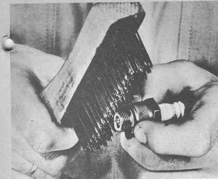
Use a petroleum solvent to remove oily fouled deposits from spark plugs. Use wire brush or rotary wire buffer to keep plug threads clean.
