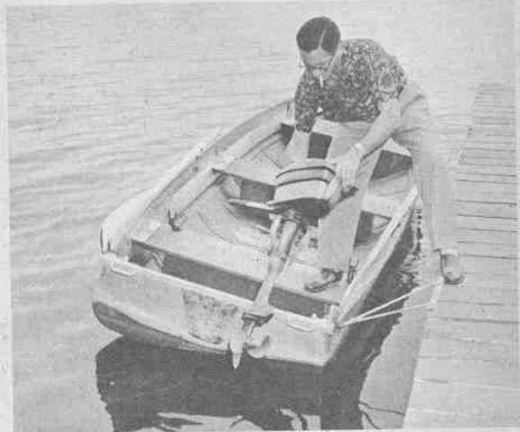
Eaton Mooring Arms steady boat while motor is being mounted.
