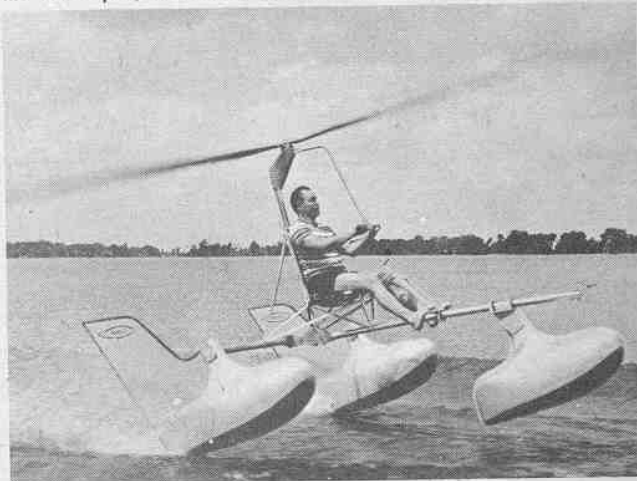
(Below) Towed behind a Mercury Mark 55 outboard motor, Hydro-Glider speeds through air, turning to right or left and climbing or diving.
