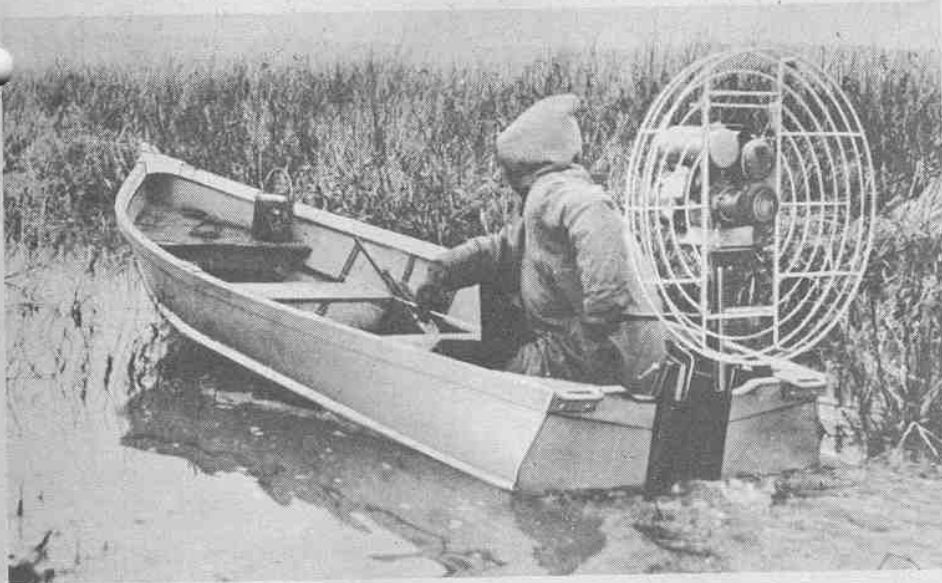
The Dragonfly Airdrive Outboard Motor, Model 80 Cruiser, has propeller 31 inches in diameter run by a 4 hp motor and can operate in very shallow waters.
