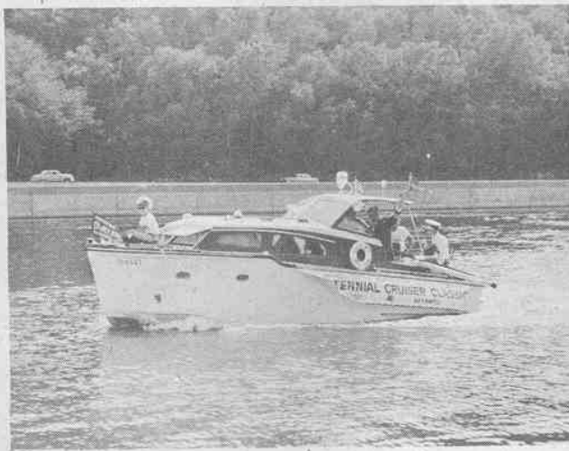
The 22-foot Nor-Craft Fiberglass outboard cruiser that ran non-stop from Minneapolis to New Orleans, powered by twin Scott-Atwater 30s.
