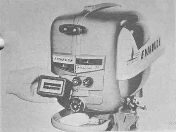
Frahm Resonant Reed Tachometer reads directly in rpm when it is held against motor housing. Two models are now available.
