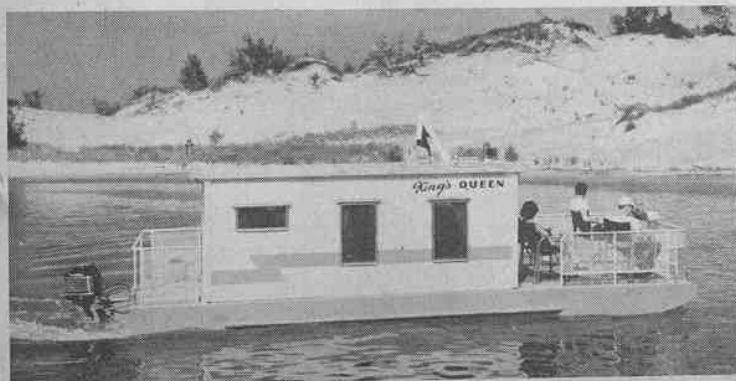
(Left) The River Queen outboard-powered houseboat has large forward deck and roomy cabin; is 24 feet long.
