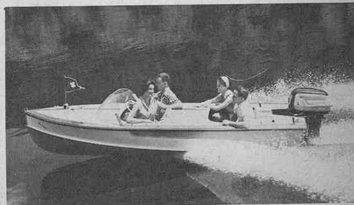
The new Chetek 15-foot Escapade, a mahogany strip-built hull, is fiberglass-covered below spray rails, has all accessories.
