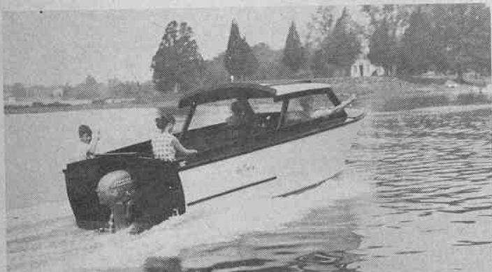
Revel Craft 20-foot Sport Cruiser has shelter cabin and a large cockpit, with metal rub rails and stem band, and water-tight motor compartment.
