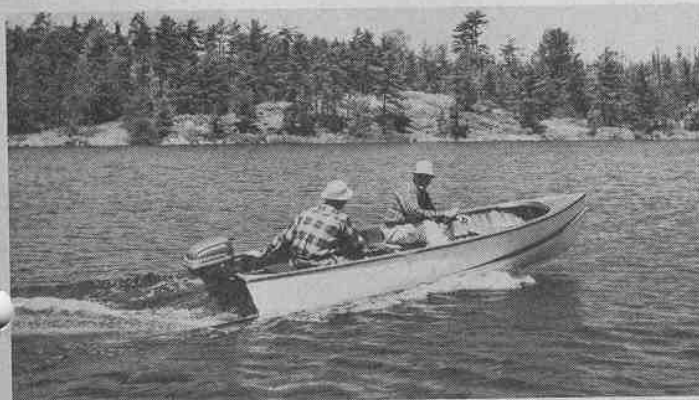
Thompson 14-foot Take-along Model 242 has canvas cover with "aqua-type" finish of plastic material; is rated for outboard motors up to 15 hp.
