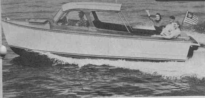
The Cruis Along Troller 22 has a hard top and a shelter cabin forward in which there are two quarter berths and room for head. Cockpit is large.
