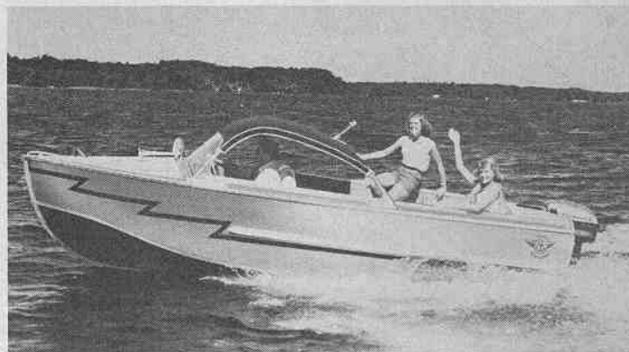
Aero-Craft Model B-18, an aluminum convertible cruiser, has remote controls, side curtains and upholstered seats; will take two large motors.
