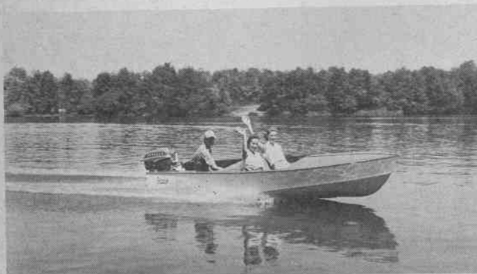
The 14-foot Model 100 Young Runabout, with center deck, is one of series of molded plywood 14-footers with various deck and cockpit arrangements.
