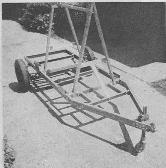
Sturdy aluminum tripod is added to completed chassis. Rubber mounting pads bolted to side rails serve as boat supports.
