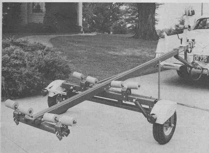
The Holsclaw Model S-150 has positive tilt mechanism that tilts and holds to desired angle.
