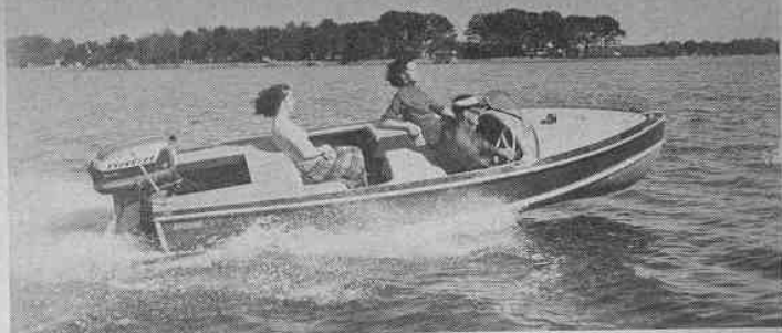
The new Whirlwind 14-foot Deluxe Runabout has hull of all mahogany molded plywood, with split center deck arrangement.
