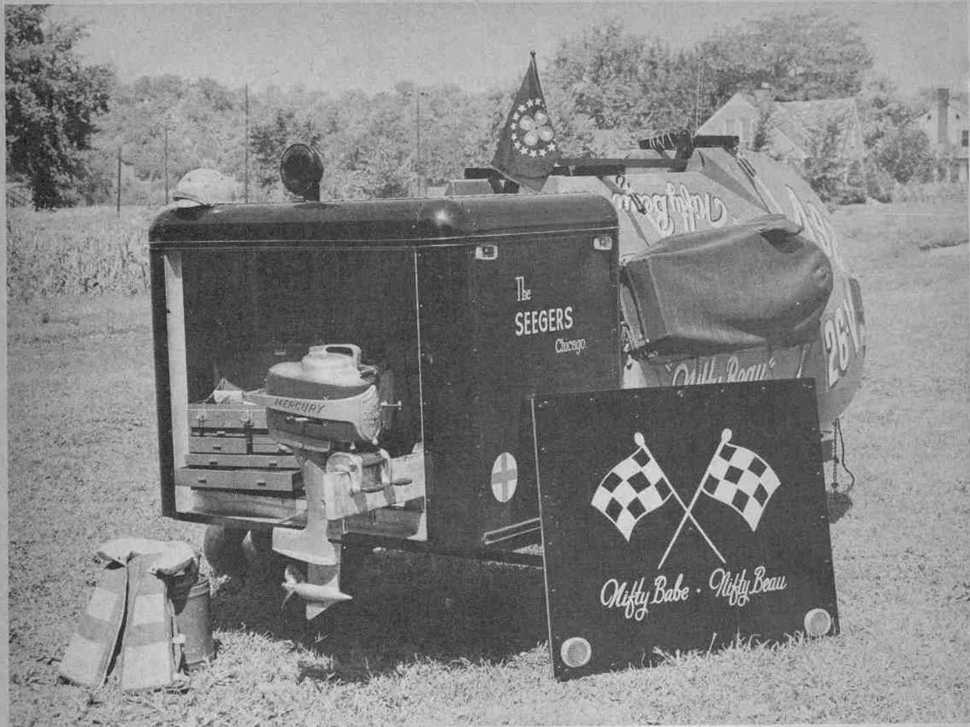
With the panel removed, the gear in the motor box is easy to get at. Aluminum brackets are on sides so that a 2" x 8" can be slipped in for motor rack. (Lower left) Cutaway drawing of motor box construction.
