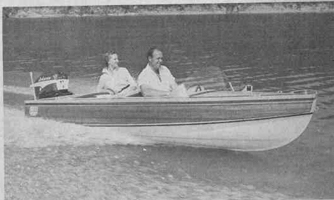
The Partee Supercraft model 14 UC has a Fiberglass-covered bottom, plexiglas wrap-around windshield, foam rubber seats.
