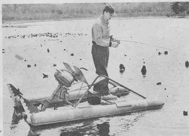
Water-Skeeter pontoon boat takes motors up to 3 hp and is hard to beat as a fishing craft in shallow, snag-filled marshes and ponds.
