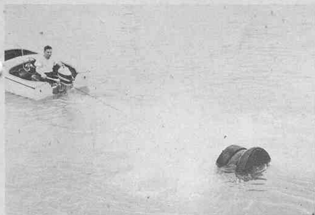
In test, fires are suspended just below the surface so that boat is not subjected to undue shock. Test is for lower unit and bracket.
