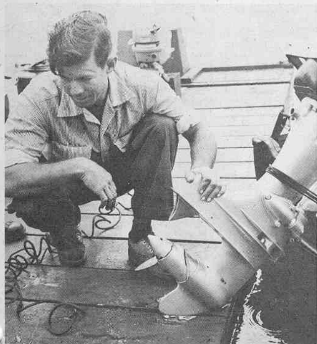
Test driver Joe Anderson inspects sheared propeller blade that temporarily interrupted testing until a replacement was put on.
