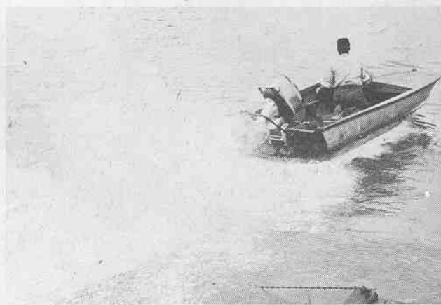
Steel-filled cables restrain the upward travel of the motor, and then it slams down against the transom with sledge hammer force.
