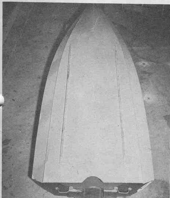
(Left) No fin is used, as it would be torn off in jumps. Oak keels, 1\frac{1}{2} " deep, put on bottom for protection, also reduce sliding.
