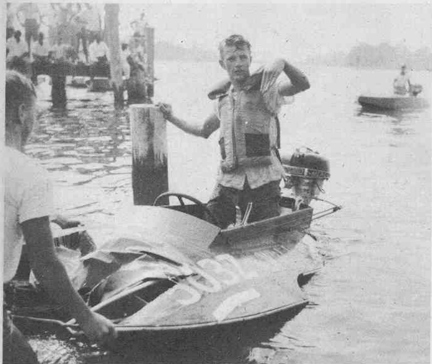
Picture taken by Bernard Abrams, Wilmington, N. C., during the A.P.B.A. Divisionals at Solomons Island, Md., shows smashed bow of a Class A stock hydro that went through wake of a cruiser. Unidentified driver (from either N. C. or S. C.) indicates how this hydro nosed down.
