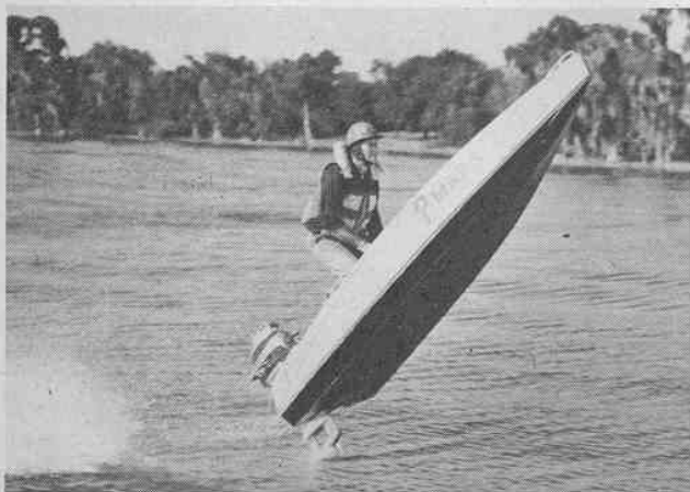
(Below) Too much weight at the stern causes boat to land this way—and maybe back-flip.
