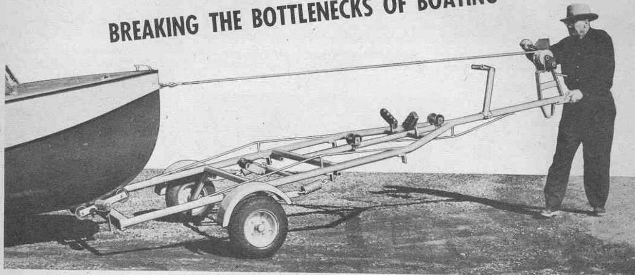
(Above) Showing the winch operation of the B. & C. Mfg. Co.'s Hilltop, Jr. model for boats up to 14' in length and weights of 450 lbs.
