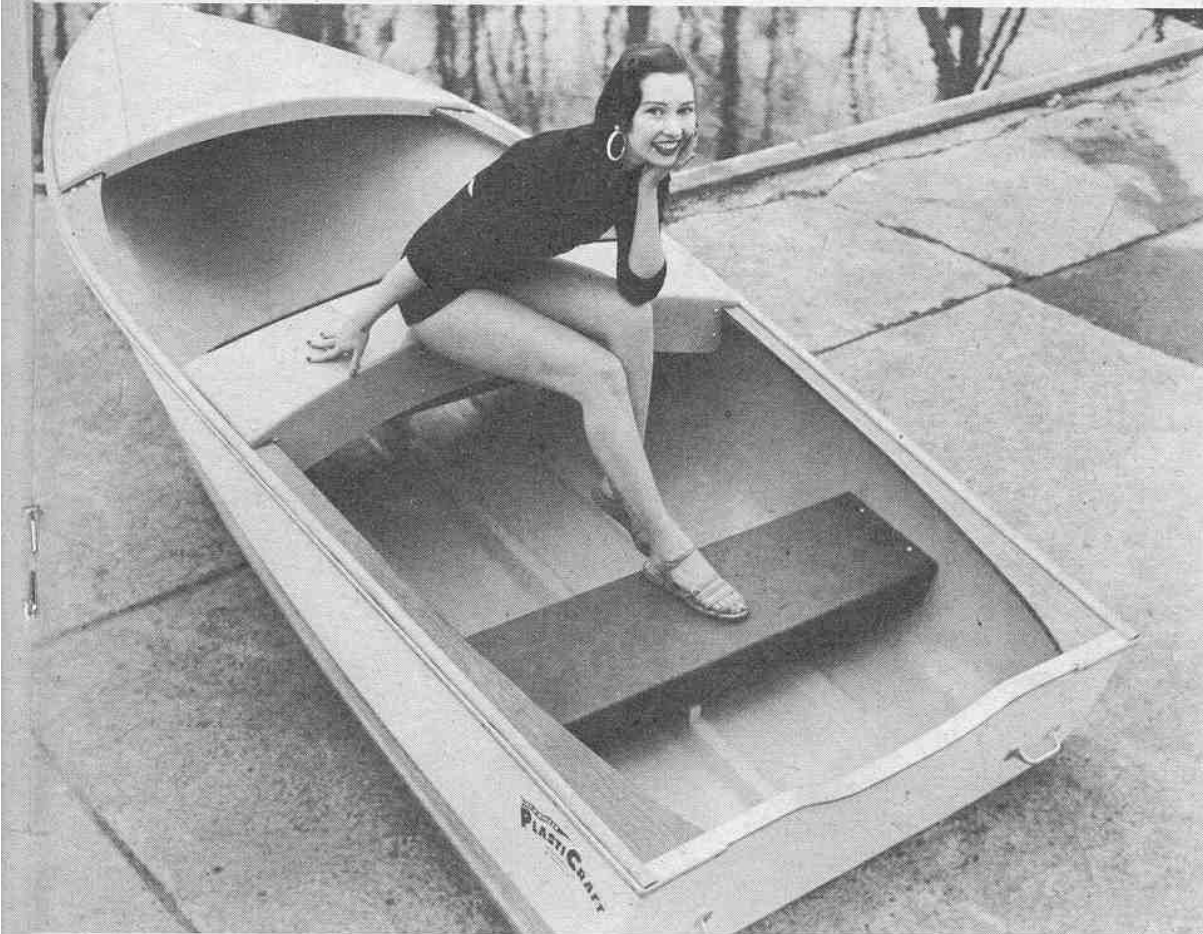
Plasti-Craft 12' runabout has a Fiberglass-reinforced plastic hull and foredeck, mahogany gunwales, ash rails.
