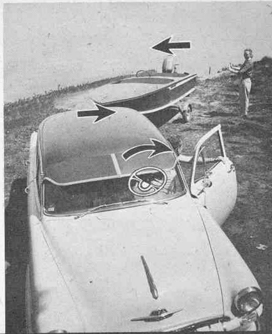
Take it easy when backing trailer into the water. Photo far left shows trailer going to the driver's left. Photo left shows how to make trailer go to driver's right. A good idea, too, is to have someone lend you a hand until you are an expert.
