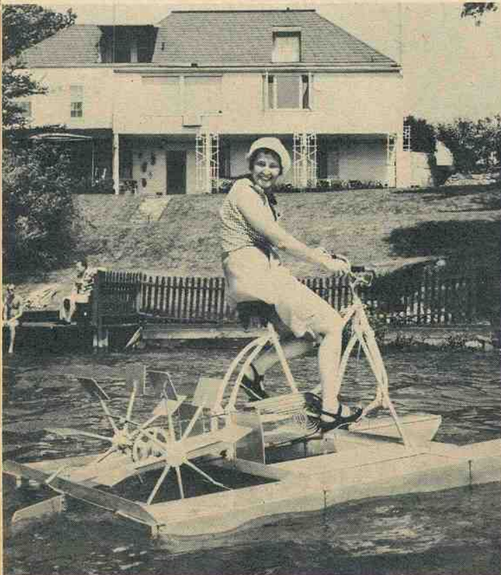
WaterBike is made by Horst Manufacturing Co., Bellville, Mich., and weighs 140 pounds. pontoons are aluminum; power is by paddle wheels.
