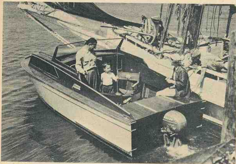
Owens Yacht Co., Inc., Baltimore 22, Md., makes a 21' outboard cruiser that sleeps three, has enclosed lavatory and head, and galley; cockpit is 6' x 9', with canopy available as an extra. Motor brackets for twin installation can be furnished. Owens 18' Sport Cruiser has a 12' open cockpit, convertible top, curtains and head. Seat converts to form a double bunk.
