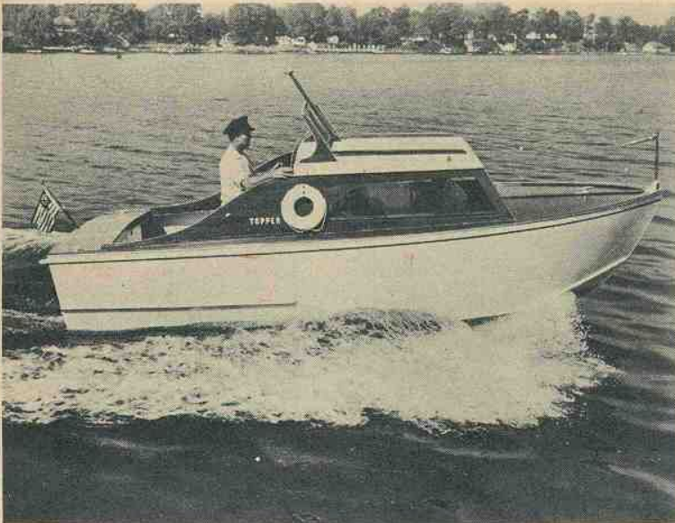
The Topper Outboard Cabin Cruiser, 19', has motor in soundproofed, water-tight compartment. Cabin has two full bunks and marine toilet. Cockpit is deep. Manufactured by the Topper Boat Co., Baltimore 25, Maryland.
