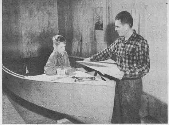
(Above) The kit boat has now been turned right side up and the deck is being fastened in place. Frame extensions have been sawed off.
