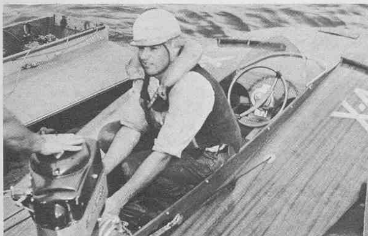
The driver of this Hadley hull has his boat equipped with spoilers on the front deck to keep the hull from becoming air-borne. Drivers unfortunately not identified.
