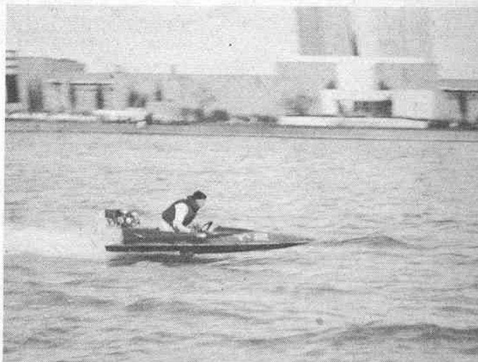
Prop riding on outboard calls for plenty of savvy on engine angles and transom heights. Smarter drivers have taken advantage of this phase of racing for a long time. Here veteran Homer Kincaid from Carbon Cliff, Ill., shows his knowledge of it with an Evinrude C during the races held at the Chicago World's Fair, back in 1933.
