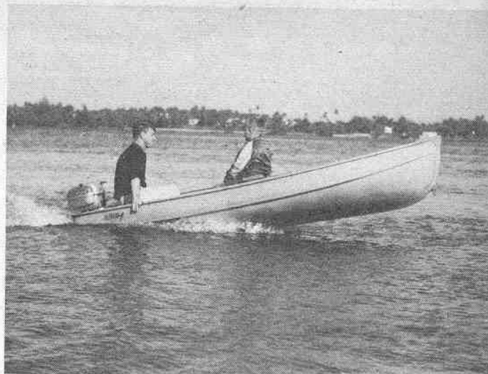
(Above) An engine tilted too far out causes a well-designed hull to mush down in the stern and point bow skyward in inefficient fashion.
