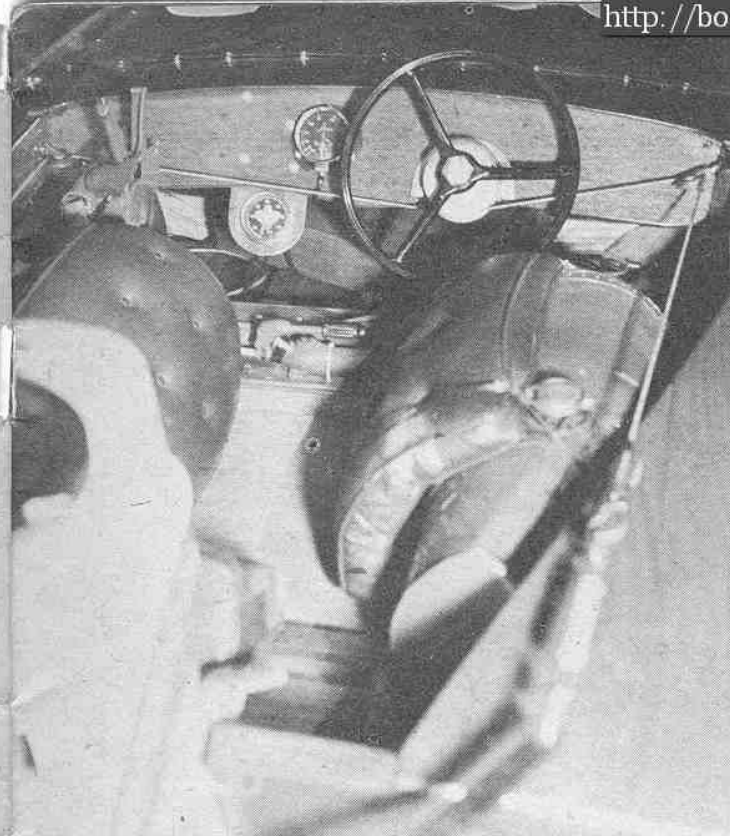
(Above) Neat, efficient cockpit of veteran marathoner Fred R. Snyder's Raveau hull. Bicycle grip under wheel operates the transom angle lift.
