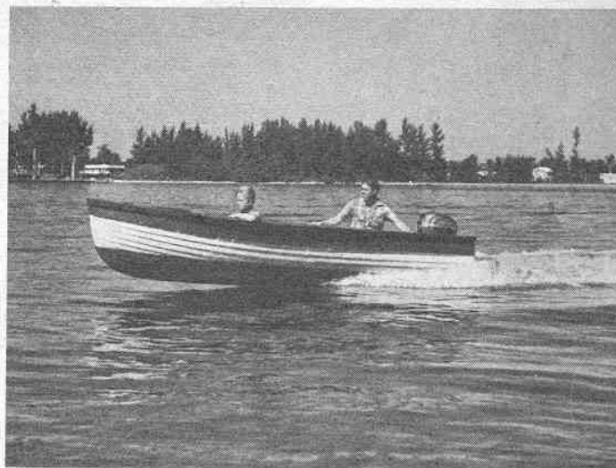
(Above) When motor is mounted at proper angle, the fore half of any well-designed runabout will plane nicely and boat will handle well.
