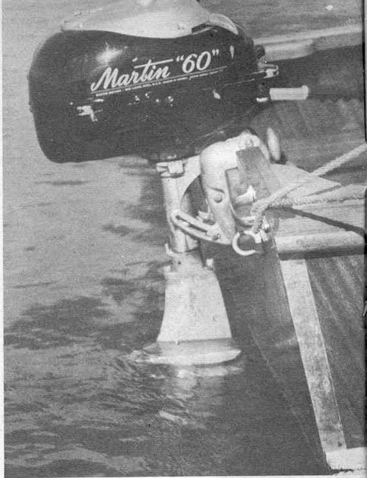
An engine mounted too close to the transom often causes a boat to be nose heavy, making it tend to fish tail and be very hard to control.
