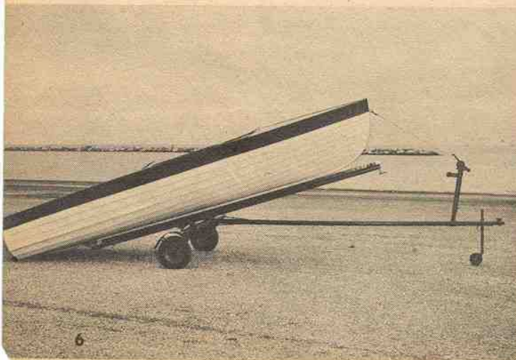
(Below) The Ace Tipper is new model in the line of Ace Iron Works of Texas. The let-down design allows the boat to slide into the water.
