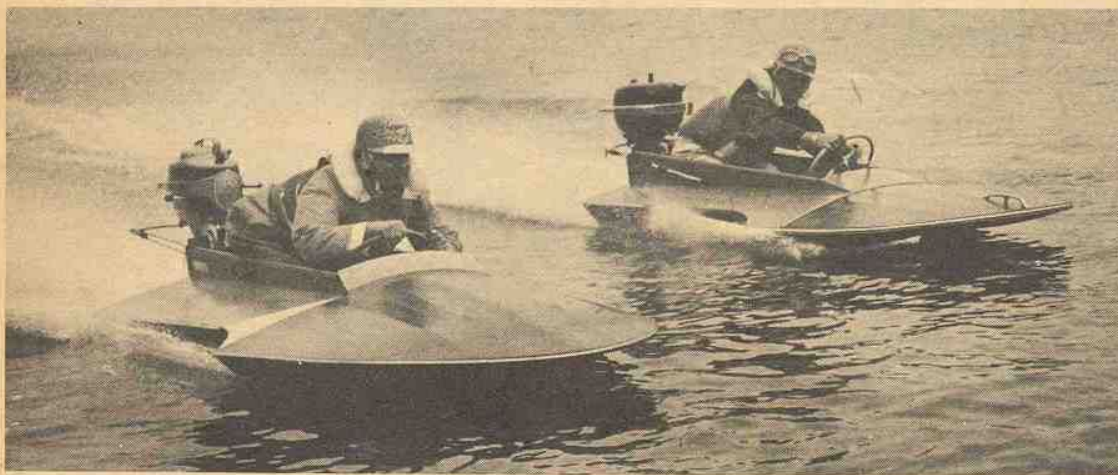
(Above) Center of gravity of new 20H is considerably lower due to use of remote fuel tank. Also note the marked profile difference between two models. KG-7H driven by Boyle, at rt., shown on Pabst hydro.
