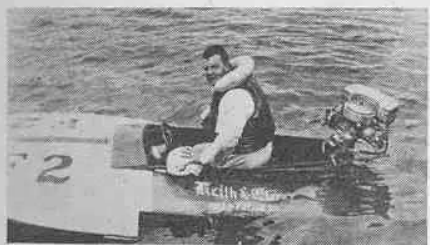
Lewis Fitzgerald of Wasilla, Alaska, the Anchorage Outboard Club's high point winner for 1953. The Fillinger three-pointer was powered by a Class C Johnson PR motor as shown here.
