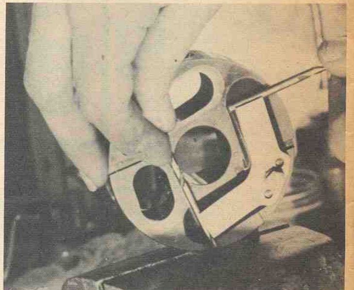
(Above) Maximum clearance between top surface of reeds to reed stops is 5/32". To check this, use 5/32" drill as a "no-go" gauge. Using one drill size smaller as "go" gauge, permits full valve limits in rules.
