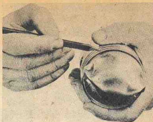
Worn file is good tool for removing ring groove carbon.
