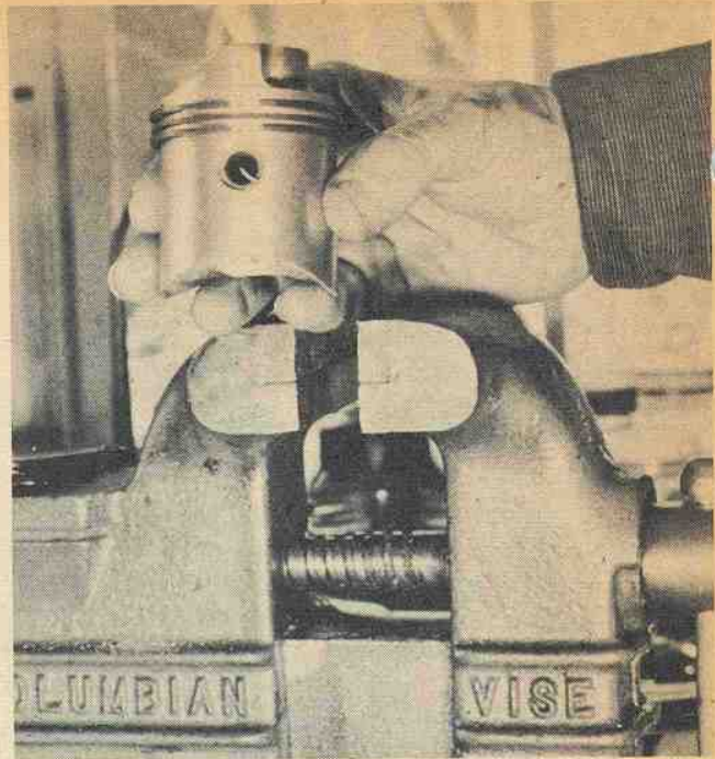
Recommended method of pinning rings is illustrated here. Each ring groove is drilled and an individual tapered retaining pin tapped into place. Note that top and bottom rings are pinned in one location—center ring, to offset blow by, is pinned on piston's opposite ends.
