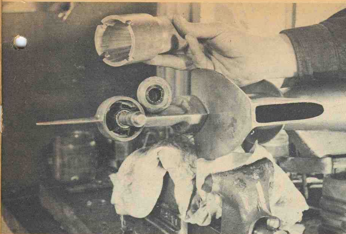
(Left) To remove the water pump cover of Quicksilver units, a special tool is required. The tool held here carries the Kiekhaefer number M-60-5146 and its cost is $7.02.
