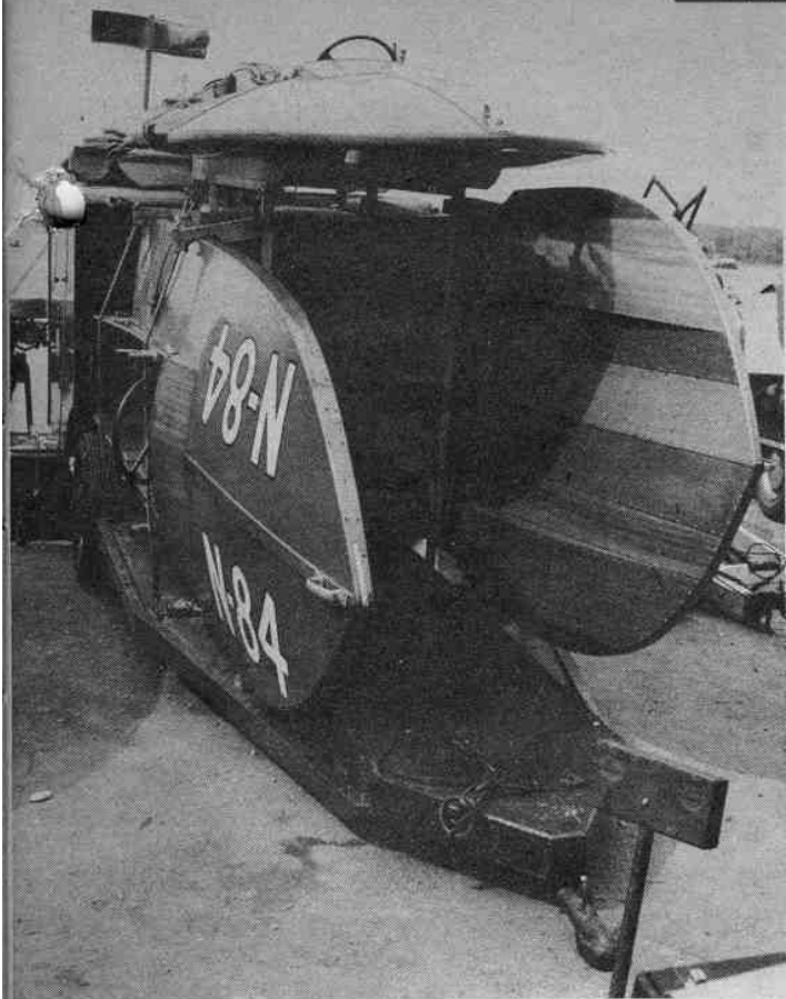
For a multi-boat set-up, hydros carried on their sides, can be compactly packed and take less of a beating on the road. Mud guards over trailer wheels (missing here) are recommended to keep road grime away from the equipment. (All photographs by H. W. Bowman)
