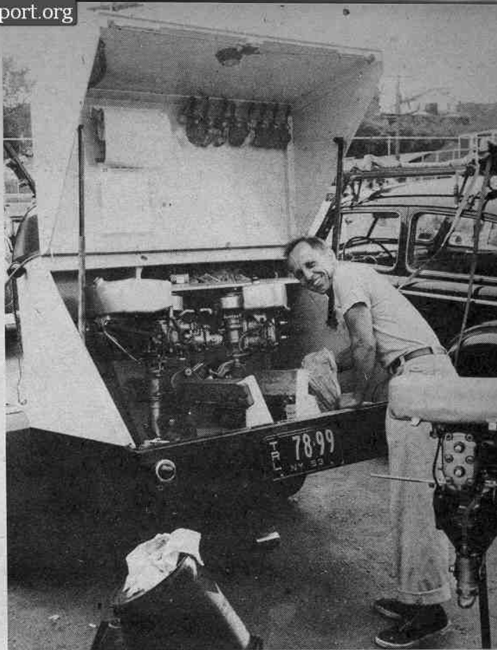
Perennially tough A and B competitor Gil Petermann, the former A champion, built this compact, well designed motor carrying box from plywood. Note overhead light above the propeller racks, a handy item for storing away equipment after dark, and paper towel roll.
