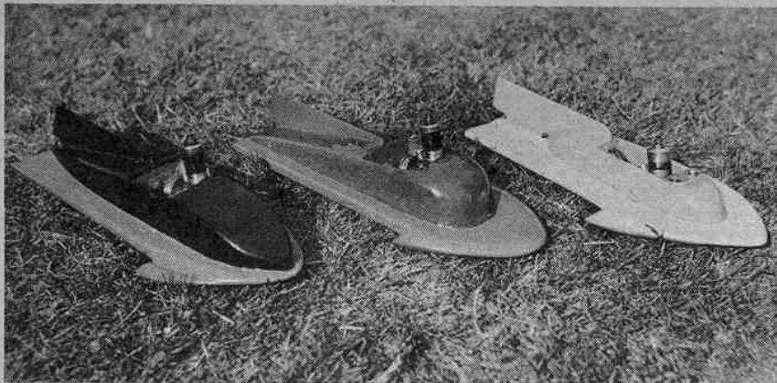
Two views (above & below) of three custom-design hydros built by the author. Main hull sections are made from solid balsa sheet, with hollow upper sections and either hollow or solid sponsons.
