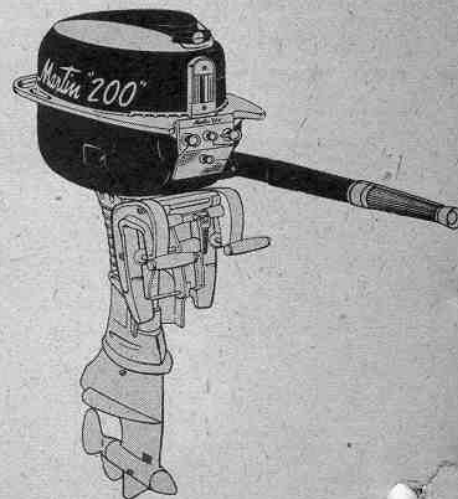
(Above) New Martin "200" Silver Liner (20 h.p.) has full gear shift, twist-grip speed and shift controls and remote auxiliary tank. Continued: "200" Silver Streak, 10 h.p. "100", 7½ h.p. "75", 4½ h.p. "45", and 2½ h.p. "20".
