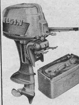
(Above) Elgin 16 h.p. has full shift, twist-grip speed control, remote tank. 7½ and 5 h.p. have neutral clutch. The 2 h.p. single is an air-cooled motor.
