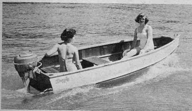
(Below) Duratech 9' aluminum pram weighs 48 lbs. Buoyancy is given by Styrofoam blocks under seats. Also Veeline runabouts, 12 and 14'
