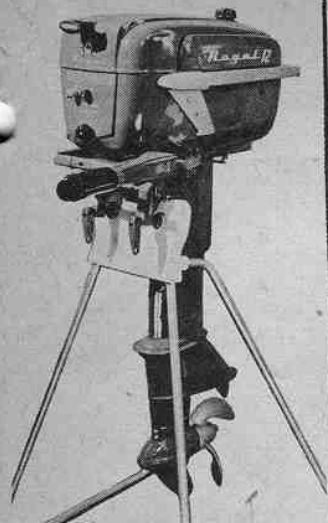
(Above) Royal 12 h.p. Deluxe has full gear shift and twist-grip speed control. Also: 3 h.p. single; 5 h.p. Standard, and 5 h.p. Deluxe with neutral clutch.
