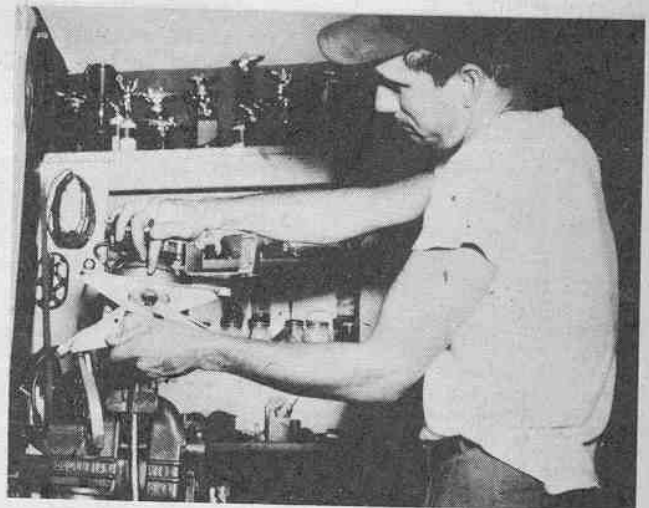
(Below) Gas tank brackets may break at point directly above the carburetor intake manifold that Larry Teal is pointing to. Broken bracket is held in left hand. Some drivers have this place bronzed under the lip.
