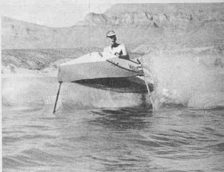
"Water Hazard V" in action! Operator has pulled back on control stick and boat has jumped until foils have left the water. When foils emerge a tremendous amount of spray is thrown as pictured here. The airplane control system feels so much like the control of aircraft that Hazard says anyone who first learns to fly one of his hydrofoils should be able to solo an airplane in less than two hours. Hydrofoils and struts are machined with 75 S.T. aluminum. All other parts can be built with minimum of machining and about one hour's welding, so Hazard tells us. Most of the parts made from common hinges. (Photo by Phil Mead).
