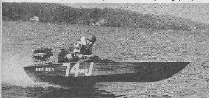
(Below) A lighter weight, four pound flywheel has added lots more snap to the already fine performance of the Mercury motor. "Dry Run" was driven in close to the shoreline at about 25 m.p.h., then the throttle was cracked wide open to show the sparkling pickup.
