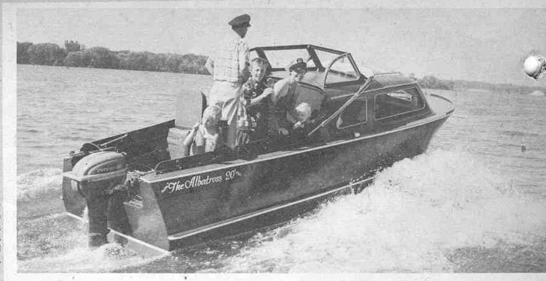
(Right) Dr. Edwin Hodge's family sets off on month's cruise from Holland, Mich., up to Mackinac. Albatross' 20' plywood hull was made by U.S. Molded Shapes, and is powered by Evinrude Big Twin.
