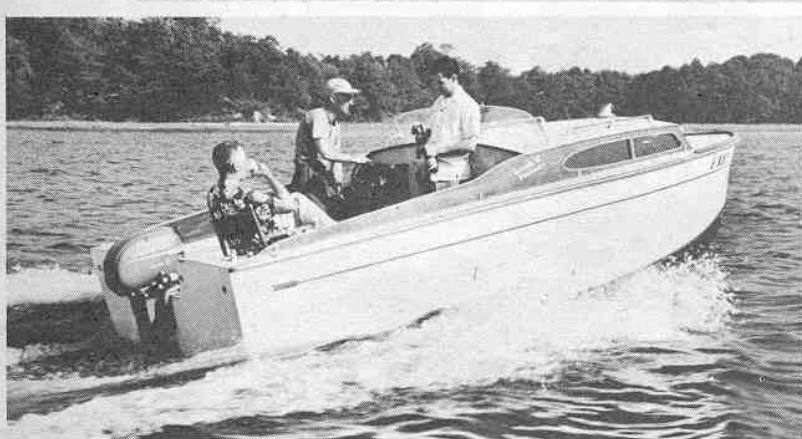
(Right) Dr. Edwin Hodge's family sets off on month's cruise from Holland, Mich., up to Mackinac. Albatross' 20' plywood hull was made by U.S. Molded Shapes, and is powered by Evinrude Big Twin.
