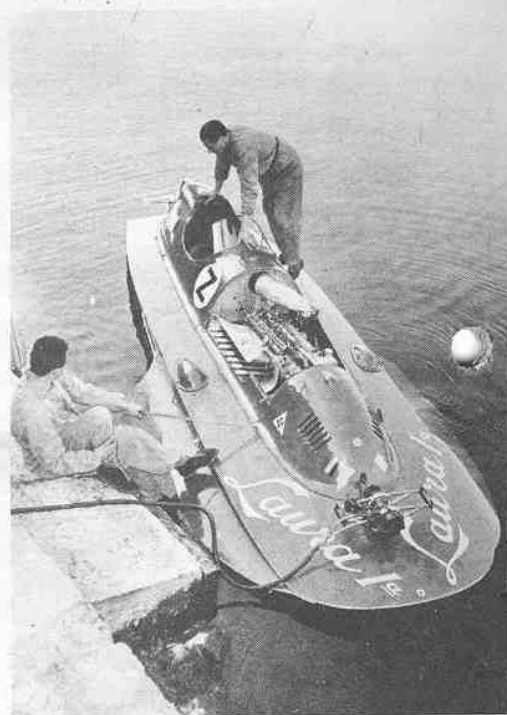
(Right) A close-up of Verga's "Laura I" shows the portable electric starter held in place near bow by electric shock cords.
