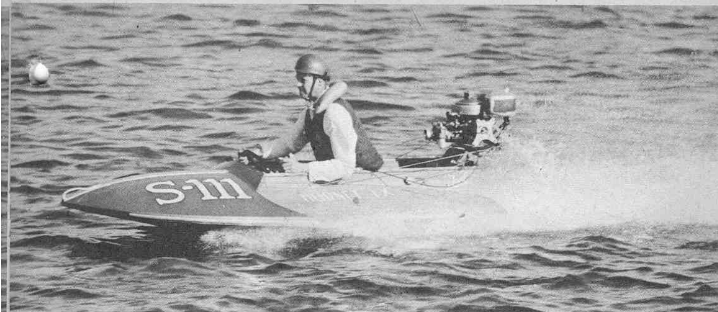
Veteran Bill Tenney set new A.P.B.A. straightaway mile record of 57.604 for Class B Outboard racing hydros—racing motors of under 20 c.i. piston displacement.
