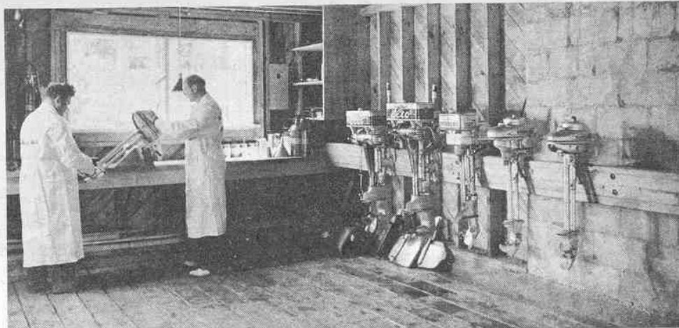
(Right) Ralph Evinrude, assisted by a mechanic, looks over a motor in a Florida test workshop. Note other motors on rack, awaiting the rigorous testing they will have to undergo for speed, durability, fuels, etc.
