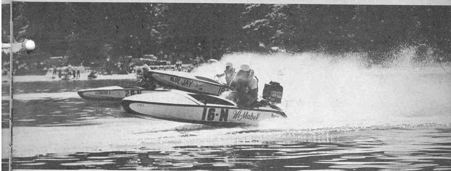
Three Raveau boats powered by Merc 25's are shown rounding a buoy in a racing event sponsored by the Stock Outboard Racing Association of Long Island at Desoris Pond, Glen Cove, N. Y. Note the variance in the handling characteristics of the three runabouts, due in all probability to variation in engine cock. Tony Rodrigues, Jamaica, in "Hi-Mabel" is pictured in the photo riding as nearly perfect as possible.
