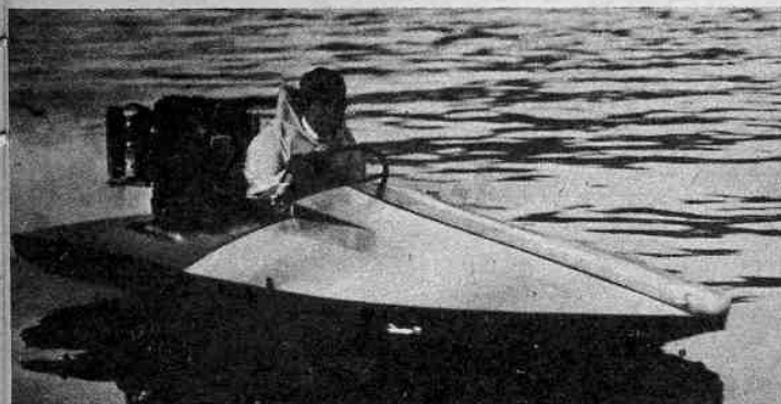
(Top, left) The four-point X boat built by the Leto brothers of Milan. Total weight about 500 lbs., it is transported by a truck and launched by crane. Like many X outfits it is powered by a privately built, modernized version of the old Spanish six-cylinder Soriano. It has 2 coaxial, counter-rotating propellers, one pusher and one tractor.
