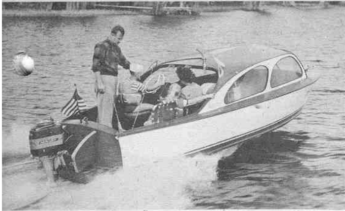
(Above) New 18' Aristo Craft cruiser has monocoque or stressed skin construction with full longitudinal mahogany stringers; sleeps three. Bracket where Mercury Mark 40 is mounted gives extra space in cockpit.
