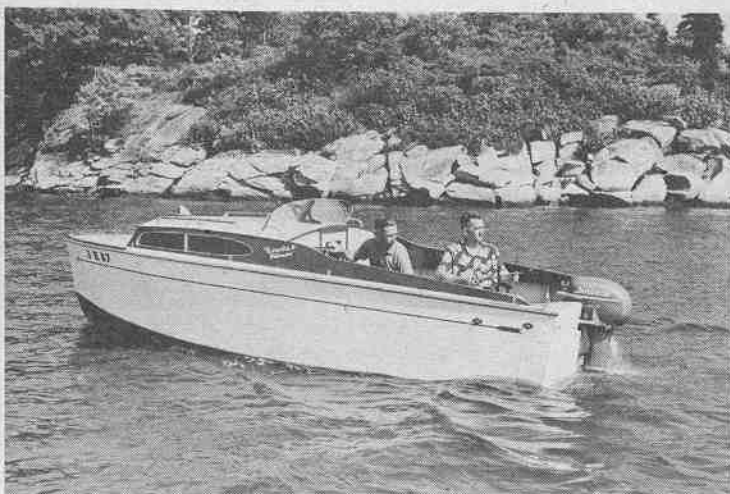
(Above) Roberts 18' Weekender, one of twelve boat kit models offered. Line includes prams, skiffs, runabouts and JU-AU stock utility racer. (Below) Aluma Craft shows first outboard cruiser—all aluminum, with berths, galley, head and buoyancy tanks. Erich Swenson is designer.
