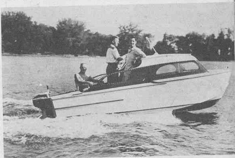
(Above) Outboard cruisers may be operated with motors from 10-50 h.p. Here 16 h.p. motor (Scott-Atwater) raises Shepard bow clear of water. (Below) Holsclaw's 1953 Boat-Roadster allows one person to put boat in water or take it out. Note that boat is underslung when carried.
