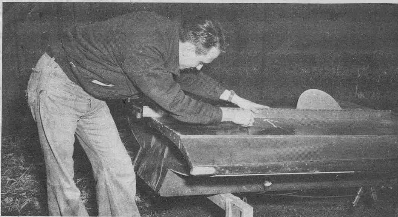
Improper storage is a major cause of a swayback formation in the planking. Watch for hooks appearing in the last 4" of the planing surface at about the transom line. Frequent checks and corrections will add miles per hour to your boat's performance. A metal or
