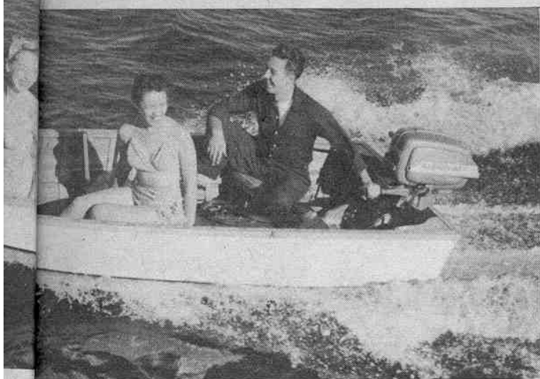
Super Fastwin planes loaded boat close to 25 m.p.h. at minimum sound level. Water-sealed exhaust and special accoustically-tuned carburetor silencer reduce noise 20% on this Evinrude 15 hp. model, which also has gear shift and twist-grip steering handle, with snap-on fixtures for the efficient Simplex remote controls.
