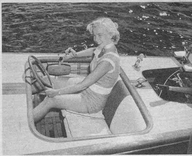
Johnson Motor's new Ship Master remote control throttle-shift unit is interchangeable on the new 10 and 25 hp. models without extra adjustment. Outer fittings on motors are standard equipment, thus avoiding drilling holes in shroud. Cables are stainless steel, rubber-sealed, to resist corrosion; in lengths 7, 9, 12 and 15 feet.
