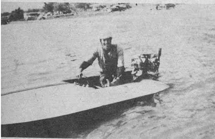
11—(Below) This is the "Draper X," on a conventional Class C Allen Smith Hydro. Notice there is no fuel tank on motor. The tank was installed forward of the steering wheel to offer better balance. Despite this precaution the boat became airborne, flipped over backwards to end my chance to break the record. That try for a record was my last experience with outboard racing. Not until 1947 did I re-enter speed-boating. I rode with Doc Novotny in "Cherub II" at Newport Beach, Cal.
