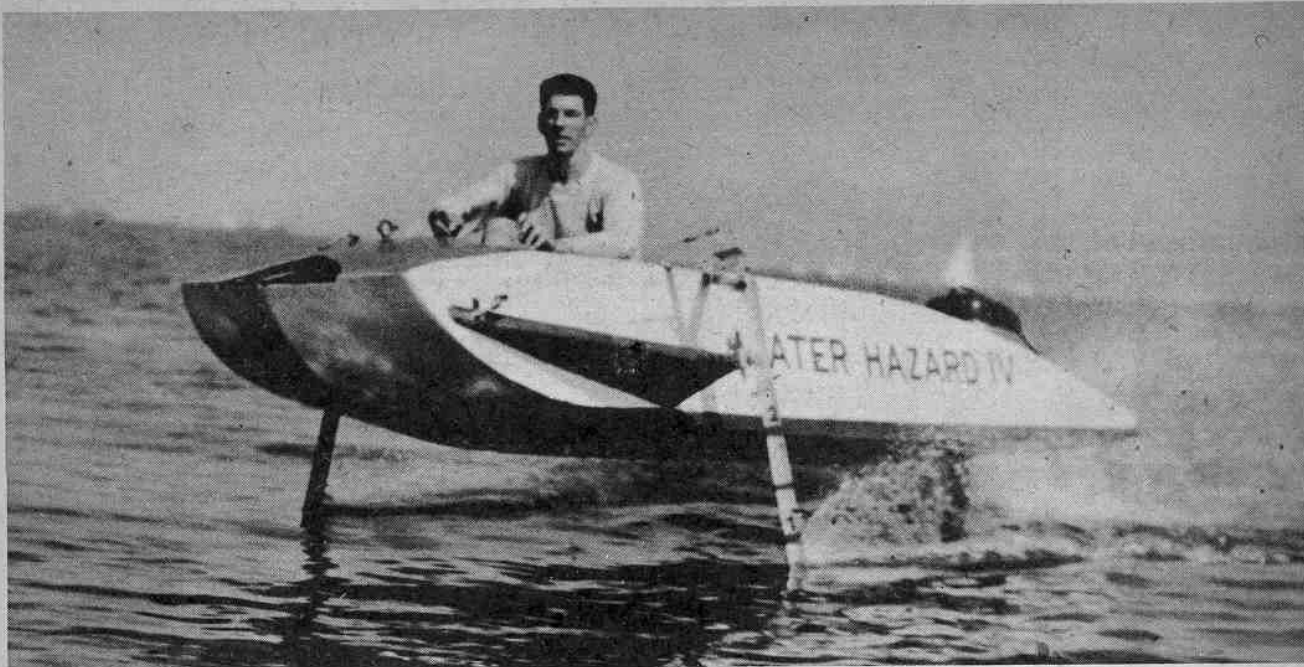
Allyn B. Hazard's Hydrofoil uses a conventional outboard runabout of blunt-nosed, sea-sled construction, powered by a Mercury motor.
