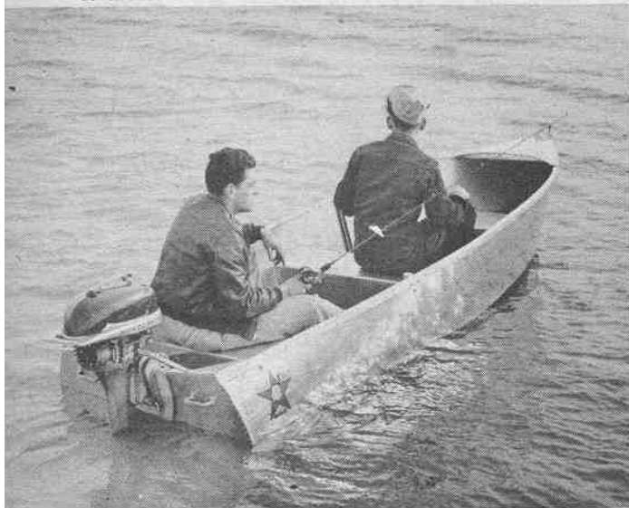
Bulkhead seats, a regular feature of most aluminum boats, are filled with Styrofoam in this 12' Blue Star Warrior to give better flotation. Special rubberized sound-deadener applied over floor eliminates early problems of metal boats. Boat weighs 90 lbs.
