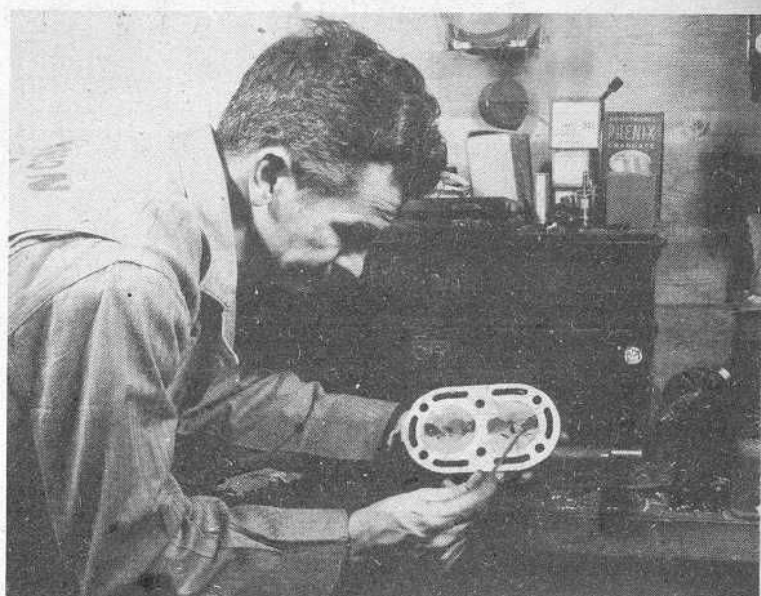
After check is made, note impression of piston in modelling clay and see also test cuts Doc Williams has made to check chamber balance. Filing away high spots from the piston crown will correct any inequalities revealed.
