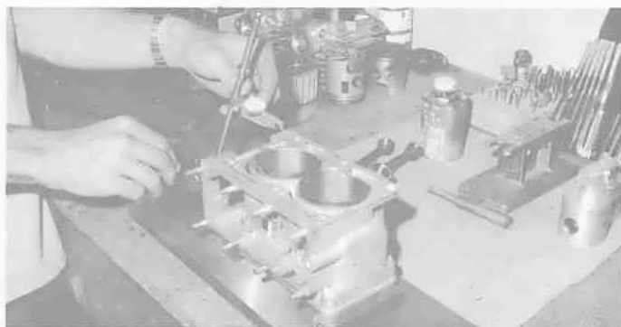
Checking to see if a Hot Rod block is square and flat
