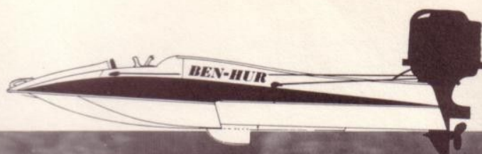
Class F Hydro with Mercury engine - speed potential: over 125 MPH
