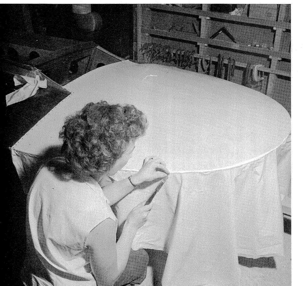
16. Fabric decking almost all tacked in position. Excess is later cut off. Remember to give this at least 6 good coats of dope, prior to painting.
