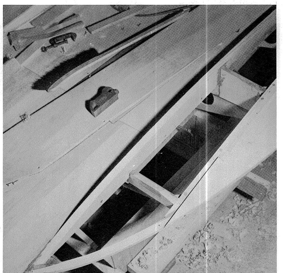
11. Planking on the side of sponson is in place and bottom has been carefully fitted. Most of the bottom planking lies over the side, but up front it butts.
